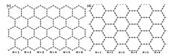
**Figure 2.** Armchair- and zigzag-edged nanoribbons can be obtained by cutting through an infinite graphyne sheet along two directions, horizontal and vertical. In (**a**,**c**), armchair-edged graphyne nanoribbons are shown with widths of N = 1 and 6, respectively, where N denotes the number of chains of carbon rings. In (**b**,**d**), zigzag-edged graphyne nanoribbons are shown with widths between N = 1 and 6. The gray and white spheres represent carbon and hydrogen atoms, respectively.
