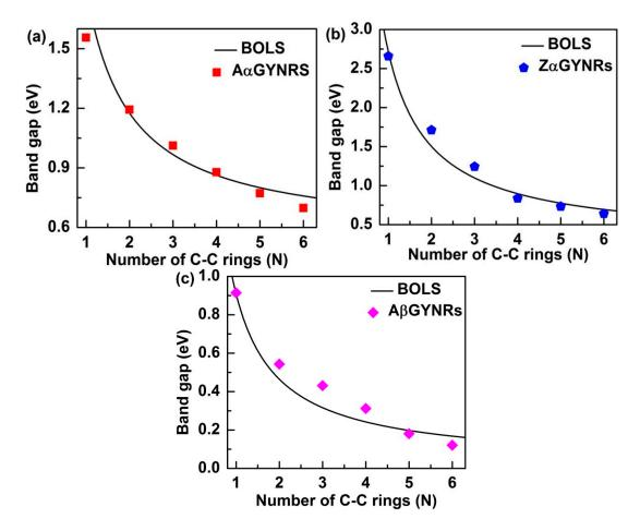
**Figure 7.** Comparison of the calculated size effect in GYNRs between ab initio and BOLS with (**a**) armchair- and (**b**) zigzag-edged  $\alpha$ -GYNRs, as well as (**c**) armchair-edged  $\beta$ -GYNRs.
