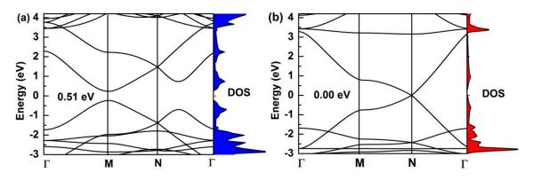
**Figure 3.** The electronic density of states and band structure for (**a**)  $\alpha$ -graphyne and (**b**)  $\beta$ -graphyne. The red and blue areas represent the electronic density of states corresponding to the band structure.
