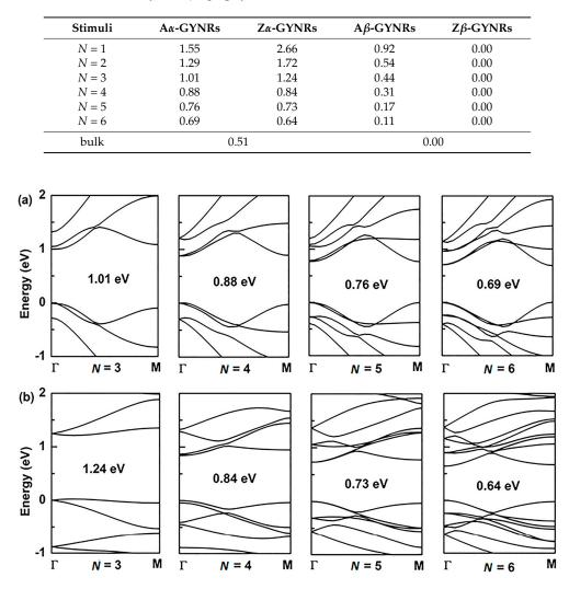
**Figure 4.** The band structure of armchair-edged  $\alpha$ -graphyne nanoribbons with (**a**) N = 3 to 6, and zigzag-edged  $\alpha$ -graphyne nanoribbons with (**b**) N = 3 to 6. The Fermi level is set to zero.
