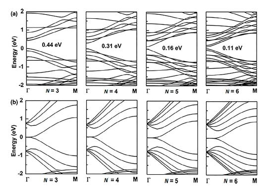
**Figure 5.** The band structure of armchair-edged  $\beta$ -graphyne nanoribbons with (**a**) N = 3 to 6, and zigzag-edged  $\beta$ -graphyne nanoribbons with (**b**) N = 3 to 5. The Fermi level is set to zero.
