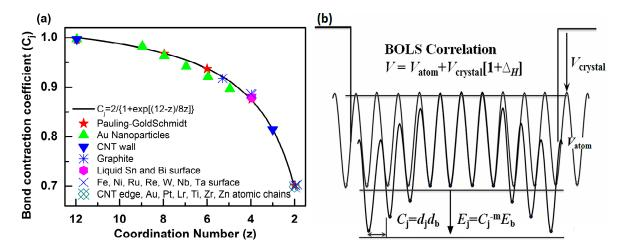
**Figure 1.** (a) The bond-order-length-strength (BOLS) approximation (solid line) represents the atomic "*CN*-radius" convention of Pauling [33] and Goldschmidt [34], with further evidence (scattered symbols) obtained from nanomaterials and surfaces; (b) Schematic illustration of broken bond-induced local strain and energy entrapment at the terminating edges, up to three atomic layers deep.
