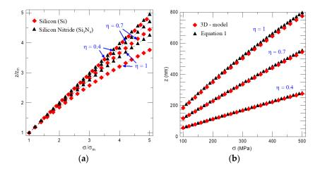
**Figure 3.** (a) Change in relative deflection  $z/z_m$  as a function of the temperature dependent tensile interlayer stress for different thickness ratios  $\eta$ ; (b) estimated static deflections of the cantilever made of Si<sub>3</sub>N<sub>4</sub> of *L* = 6 µm, *W* = 900 nm and *T*<sub>1</sub> = 250 nm for three different NiTi film thicknesses as a function of the temperature dependent interlayer stress calculated by Equation (1) and the 3D model.
