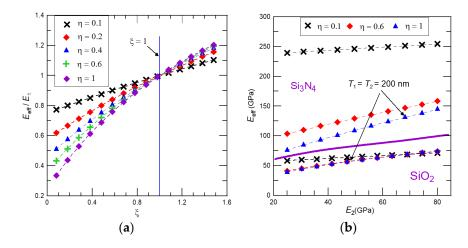
**Figure 2.** (a) Variation of the relative effective Young's modulus of the cantilever, i.e.,  $E_{\text{eff}}/E_{\text{s}}$ , as a function of the temperature-dependent NiTi film Young's modulus represented through the dimensionless modulus ratio  $\xi$  for different thickness ratios  $\eta$ ; and (b) the cantilever effective Young's modulus as a function of the NiTi thin film modulus for two different substrate materials, SiO<sub>2</sub> and Si<sub>3</sub>N<sub>4</sub>.
