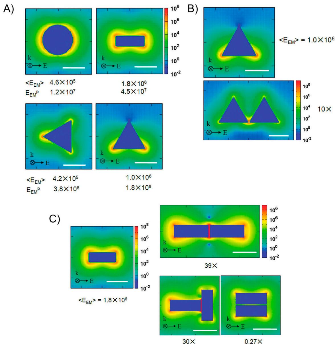
**Figure 8.** The contours of  $E_{EM}$  obtained from the DDA calculations. (A) The isolated particles: a circular disk, triangular prisms for two orientations, and a cylindrical rod with no end caps; (B) a dimer of triangular prisms with a 2-nm gap; (C) dimers of rods with 2-nm gaps: (1) head-to-head, (2) perpendicular, and (3) side-by-side. Reproduced with permission from Reference [104]. Copyright American Chemical Society, 2012.
