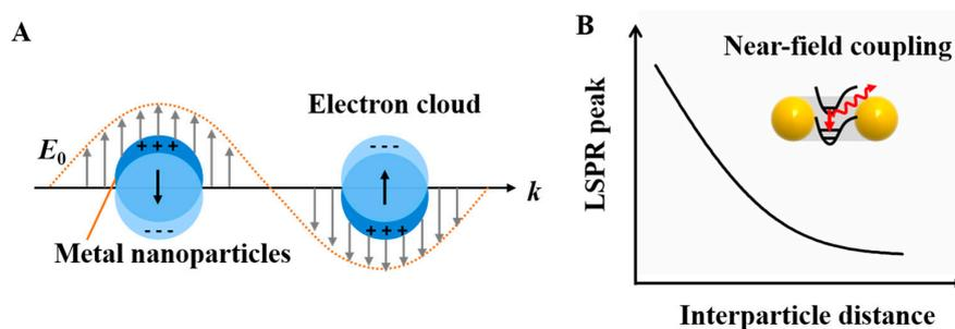
**Figure 3.** (A) The schematic of the plasmon oscillation for metal nanoparticles showing the displacement of the conduction electron charge cloud relative to the nuclei. (B) Localized surface plasmon resonance near the field coupling of the NPs dimers correlated with the interparticle distance.
