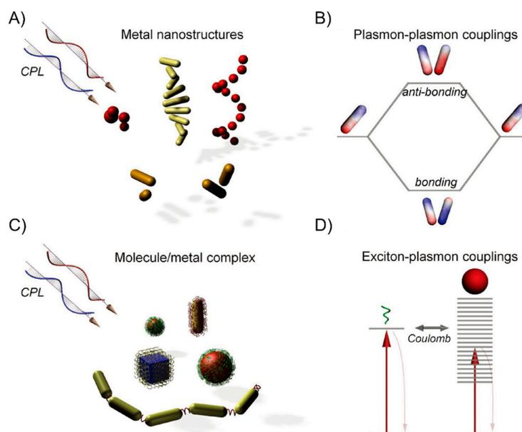
**Figure 5.** The representative physical principles involved in the chiral plasmonic nanostructures under circularly polarized light (CPL): plasmon–plasmon coupling (A,B) and exciton–plasmon coupling (C,D). Reproduced with permission from Reference [69]. Copyright John Wiley & Sons, Inc., 2016.
