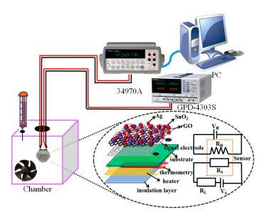
Figure 2. Schematic of the acetylene sensing experimental setup.
