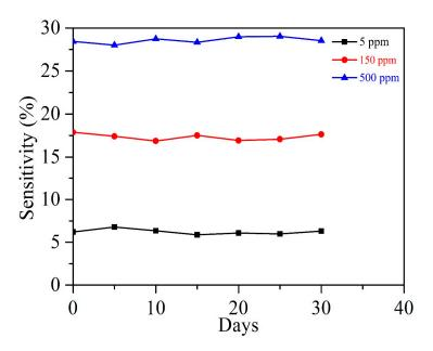
**Figure 9.** Long-term stability of the Ag– $SnO_2/rGO$  nanocomposite film sensor, measured every five days for over 30 days.
