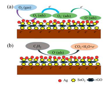
**Figure 11.** The sensing mechanism of the  $Ag-SnO_2/rGO$  nanocomposite film in (**a**) air and (**b**) acetylene gas.
