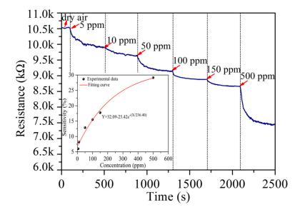
**Figure 6.** Resistance measurement of the Ag–SnO<sub>2</sub>/rGO nanocomposite film sensor upon exposure to acetylene gas with cumulated concentrations at 90 °C.
