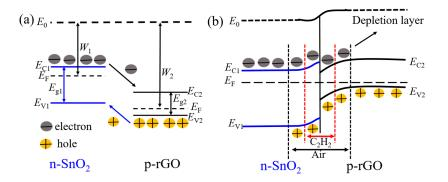
**Figure 12.** Schematic of the energy band diagram and the variation in depletion layer thickness for the  $SnO_2/rGO$  heterojunction. ( $E_C$ , conductor band;  $E_g$ , band gap;  $E_V$ , valence band;  $E_F$ , Fermi level; W, work function)
