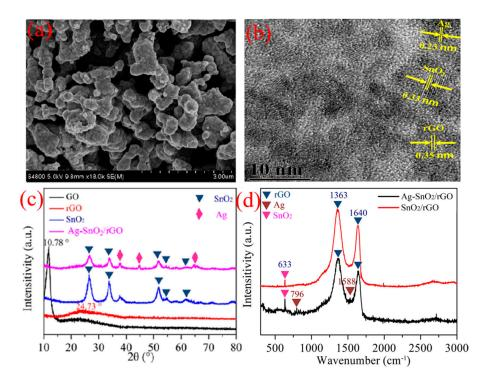
**Figure 3.** (a) SEM characterization of the Ag–SnO<sub>2</sub>/rGO nanocomposite, (b) TEM image of the Ag–SnO<sub>2</sub>/rGO nanocomposite, (c) XRD spectrum of GO, rGO, SnO<sub>2</sub> and the Ag–SnO<sub>2</sub>/rGO nanocomposite, (d) Raman spectrum of the SnO<sub>2</sub>/rGO and Ag–SnO<sub>2</sub>/rGO nanocomposites.
