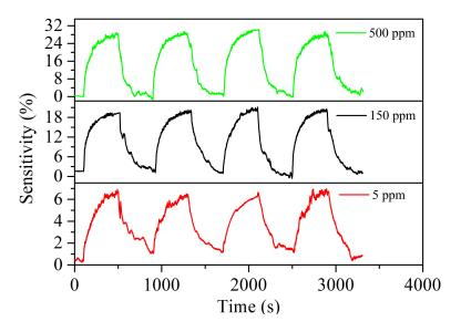
**Figure 7.** Repeatability of the Ag–SnO<sub>2</sub>/rGO nanocomposite film sensor toward acetylene concentrations of 5, 150 and 500 ppm at 90  $^{\circ}$ C.
