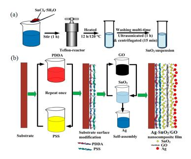
**Figure 1.** (a) Hydrothermal synthesis of  $SnO_2$  and (b) layer-by-layer self-assembly of the Ag- $SnO_2$ /GO nanocomposite film.
