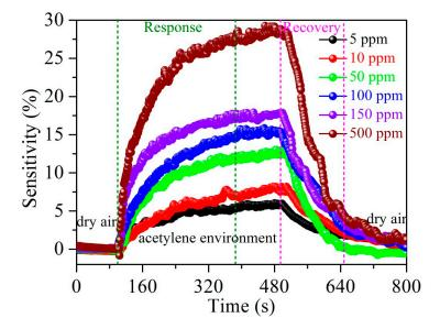
**Figure 8.** Typical response and recovery curves of the Ag–SnO<sub>2</sub>/rGO nanocomposite film sensor to acetylene pulses between 0 and 500 ppm.
