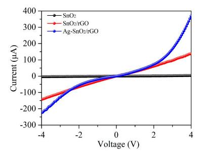
Figure 10. The measured I–V curves of the SnO<sub>2</sub>, SnO<sub>2</sub>/rGO and Ag–SnO<sub>2</sub>/rGO films.
