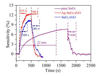
**Figure 5.** The sensitivity of pure  $SnO_2$ ,  $SnO_2/rGO$  and  $Ag-SnO_2/rGO$  film sensors to 50 ppm acetylene at 90 °C.
