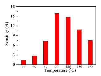
**Figure 4.** The sensitivity of the Ag–SnO<sub>2</sub>/rGO nanocomposite sensor to 100 ppm acetylene under different operating temperatures.
