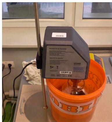
**Figure 2.** Laboratory stand for the production of the CNT suspension.
