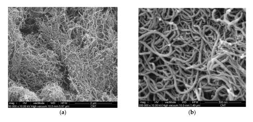
Figure 1. SEM images of carbon nanotubes (CNTs) used: (a) magnification 50,000×; (b) magnification 200,000×.
