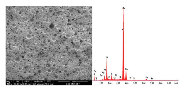
**Figure 11.** EDS spectra of series C52CNT with w/c = 0.4 together with the SEM image of the analyzed area.
