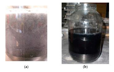
**Figure 3.** The CNT water suspension: (**a**) before sonication—visible clusters of CNT in the form of "lumps"; (**b**) after sonication—uniform color of the suspension, which indirectly correspond to a uniform CNT dispersion.
