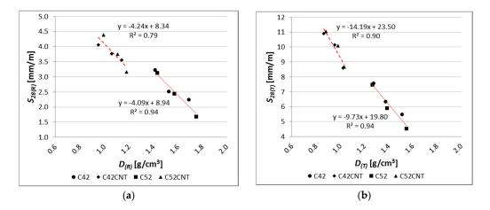
**Figure 14.** Relationship between linear shrinkage and apparent density of tested materials for (a) reference samples; (b) samples after thermal load.
