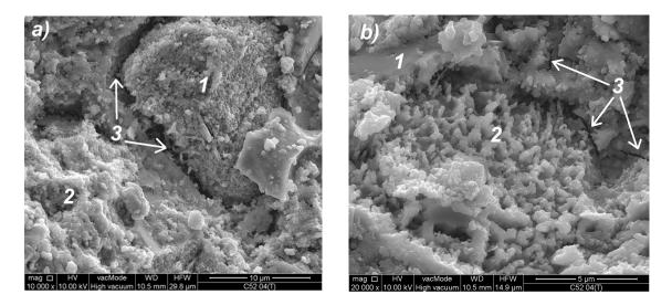
**Figure 17.** SEM photos of the C52 cement paste microstructure (descriptions of the indications in the text) for (**a**) magnification  $10,000 \times$ ; (**b**) magnification  $20,000 \times$ .
