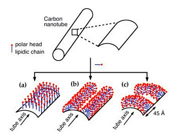
**Figure 12.** Different possible organizations of the SDS molecules on the surface of a CNT: (a) perpendicular adsorption; (b) half-cylinders oriented parallel to the tube axis; (c) half-cylinders oriented perpendicular to the tube axis [47]. Reproduced with permission of [47]. Copyright AAAS, 2003.
