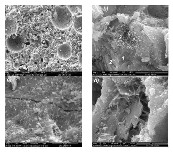
**Figure 18.** SEM photos of the C52CNT cement paste microstructure (descriptions of the indications in the text) for (**a**) magnification  $1000 \times$ ; (**b**) magnification  $25,000 \times$ ; (**c**) magnification  $20,000 \times$ ; (**d**) magnification  $40,000 \times$ .
