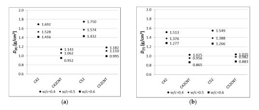
**Figure 4.** Apparent density of modified cement pastes (error bars mean standard deviations of apparent density; due to the very small values, the error bars are invisible) for (**a**) reference samples; (**b**) samples after thermal load.
