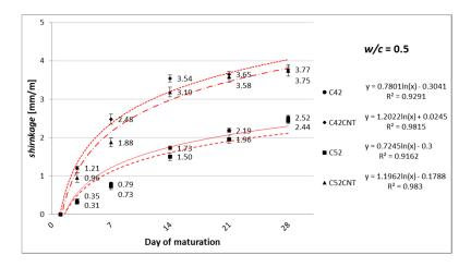
**Figure 6.** Increase in linear shrinkage of modified cement paste with w/c = 0.5, as a function of maturation time.
