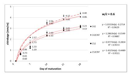
**Figure 7.** Increase in linear shrinkage of modified cement paste with w/c = 0.6, as a function of maturation time.
