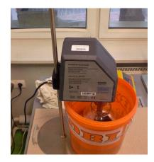
Figure 2. Laboratory stand for the production of the CNT suspension.
