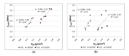
**Figure 16.** Relationship between bending tensile strength and apparent density of tested materials for (a) reference samples; (b) samples after thermal load.
