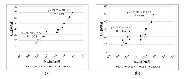
**Figure 15.** Relationship between compressive strength and apparent density of tested cement pastes for (**a**) reference samples; (**b**) samples after thermal load.
