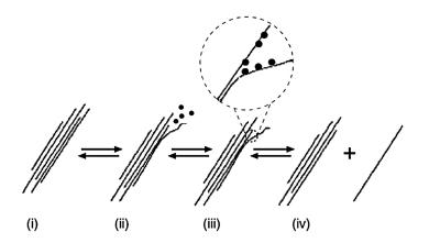
**Figure 13.** Mechanism of nanotube isolation from bundle obtained by sonication and surfactant stabilization: (i) nanotubes bundle; (ii) providing high local shear by sonication; (iii) surfactant adsorption; (iv) separation of the individual nanotube from the bundle [48]. Reproduced with permission of [48]. Copyright American Scientific Publishers, 2003.
