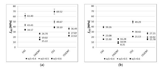
**Figure 8.** Compressive strength of modified cement pastes (error bars mean standard deviations of compressive strength) for (**a**) reference samples; (**b**) samples after thermal load.
