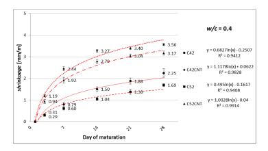
**Figure 5.** Increase in linear shrinkage of modified cement paste with w/c = 0.4, as a function of maturation time.
