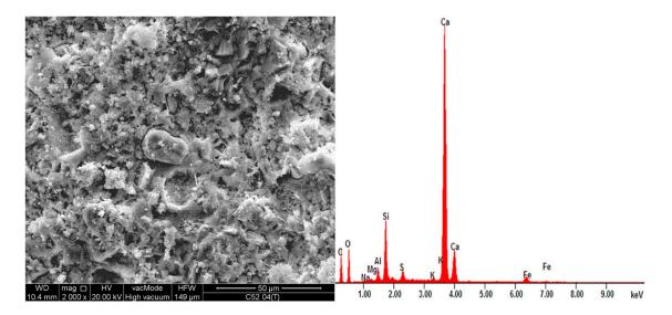
**Figure 10.** EDS spectra of series C52 with w/c = 0.4 together with the SEM image of the analyzed area.
