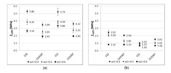
Figure 9 shows the flexural strength of all tested cement paste series.
