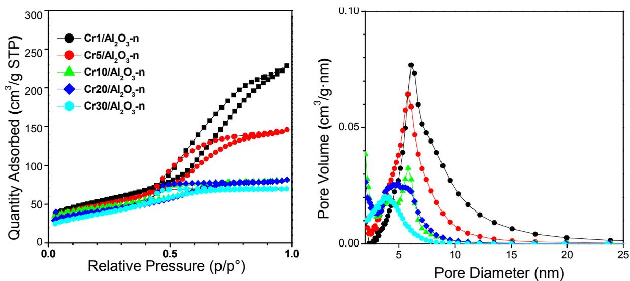
**Figure S3.** N<sub>2</sub> adsorption-desorption isotherms of Cr<sub>x</sub>/Al<sub>2</sub>O<sub>3</sub>-n catalysts.
