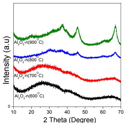
**Figure S2.** XRD patterns of alumina samples calcined at 600, 700, 800 and 900 °C.
