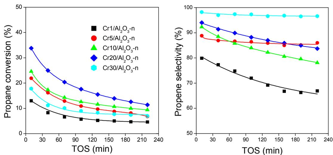
Figure S5. Variation of propane conversion and selectivity to propylene with time-on-stream (TOS) over Cr<sub>x</sub>/Al<sub>2</sub>O<sub>3</sub>-n catalysts with different Cr<sub>2</sub>O<sub>3</sub> content. Dehydrogenation conditions: reaction temperature = 550 °C; catalysts weight = 200 mg; feed gas composition C<sub>3</sub>H<sub>8</sub>:He = 1:14; total flow rate = 30 cm<sup>3</sup>·min<sup>-1</sup>.
