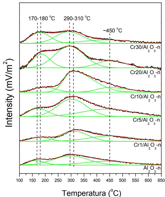
Figure S4. NH<sub>3</sub>-TPD profiles of pure Al<sub>2</sub>O<sub>3</sub>-n (calcined at 700 °C) and Cr<sub>x</sub>/Al<sub>2</sub>O<sub>3</sub>-n catalysts.
