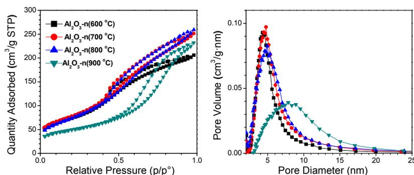
**Figure S1.** N<sub>2</sub> adsorption–desorption isotherms of alumina samples calcined at 600, 700, 800 and 900 °C.
