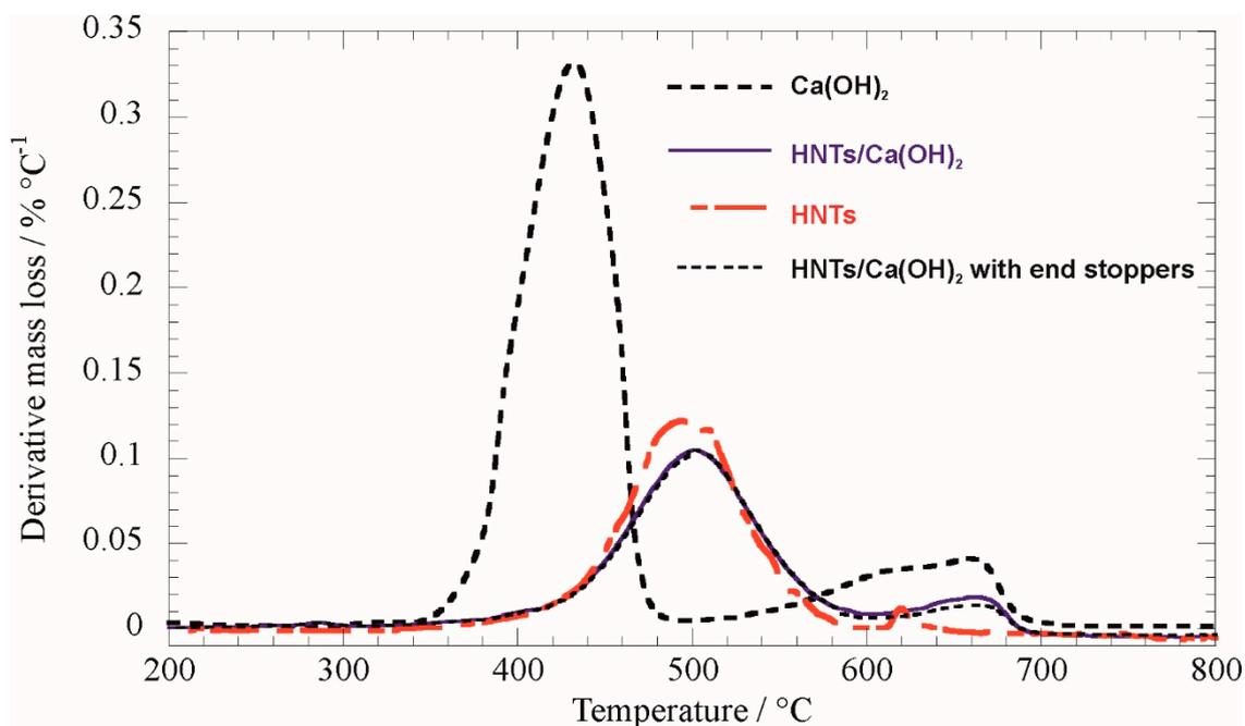
**Figure S1.** DTG curves for HNTs, Ca(OH)<sub>2</sub>, HNTs/Ca(OH)<sub>2</sub>, and HNTs/Ca(OH)<sub>2</sub> with end stoppers.
