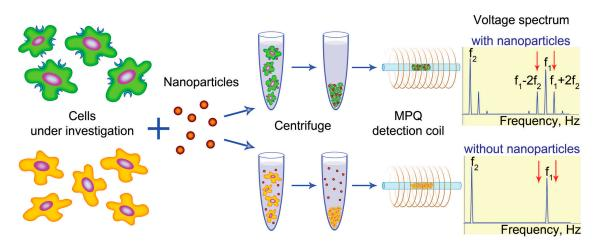
**Figure 4.** Schematic of the magnetic particle quantification (MPQ)-cytometry workflow. The investigated cells are incubated with the suspended nanoparticles. The unbound nanoparticles are then removed from the sample by centrifugation. The amount of nanoparticles bound to the cells is measured using the magnetic particle quantification (MPQ) technique at combinatorial frequencies (Reproduced with permission from [38]. The Royal Society of Chemistry, 2016.).
