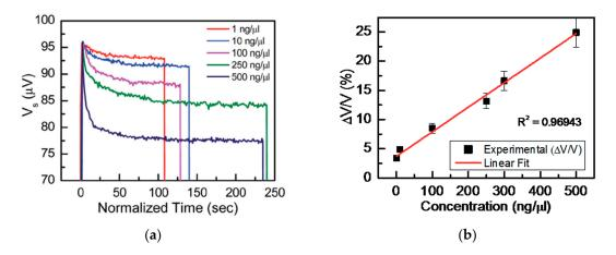
**Figure 3.** (a) Change in the sensor voltage with accumulation of superparamagnetic Nanomag-D beads on the micro-conductor with respect to the normalized time (*t* assumed zero at the beginning of the measurement); (b) Relative change in the voltage across the GMR sensor head due to the presence of various concentrations of Nanomag-D beads on the microconductor (MC) (Reproduced with permission from [36]. The Royal Society of Chemistry, 2015.).
