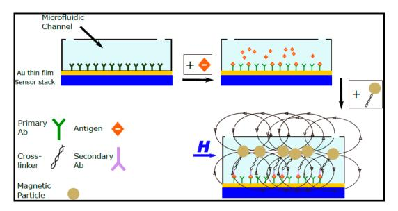
Figure 1. Schematic of the working principle of a standard magnetic biosensor.
