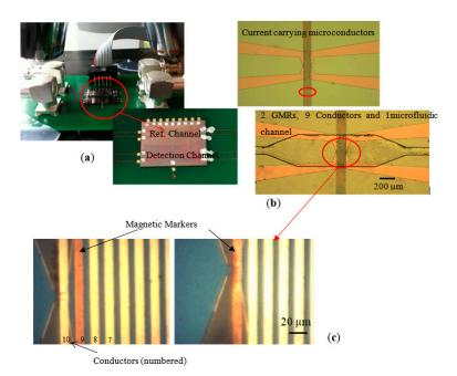
**Figure 2.** (a) The developed biosensor that consists of the giant magnetoresistance (GMR) sensors, the microconductors and the microfluidic channels; (b) Microscope image of the microconductors and a microfluidic channel; (c) Detailed image of the microconductors and the GMR sensor with magnetic markers as they moved from the right to the left microconductor.
