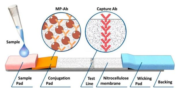
**Figure 5.** Schematic of a test strip based on sandwich-lateral flow assay with antibody-conjugated magnetic particles as labels (Reproduced with permission from [39]. ACS Publications, 2016.).
