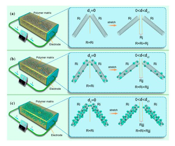
Figure 7. Schematic sensing models of sensors: (a) CNTs, (b) Ag@CNTs1, and (c) Ag@CNTs2.
