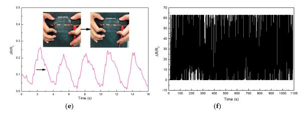
**Figure 8.** Body movement sensing of (**a**) arm motion detection results of rotation; (**b**) wrist bending; (**c**) motion detection results of elbow bending; (**d**) heart beat; (**e**) breath; (**f**)  $\Delta R/R_0$  as a function of multiple stretching and releasing cycles with 22% strain for Ag@CNTs1-based sensor.
