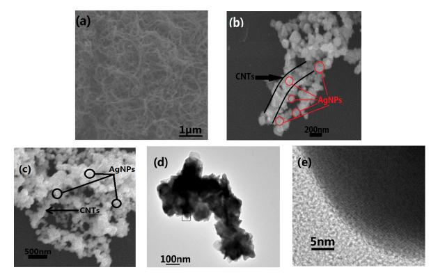
Figure 4. (a) SEM image of CNTs; (b) SEM image of Ag@CNTs1; (c) SEM image of Ag@CNTs2; (d) TEM; and (e) HRTEM images of Ag@CNTs1.
