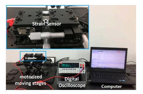
Figure 2. The strain sensing measurement platform.
