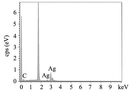
Figure 3. EDS spectrum of Ag@CNTs.
