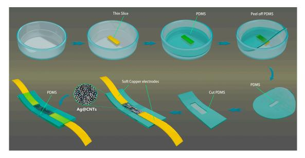
Figure 1. Schematic of the structural design and fabrication process flowchart of the sensor.
