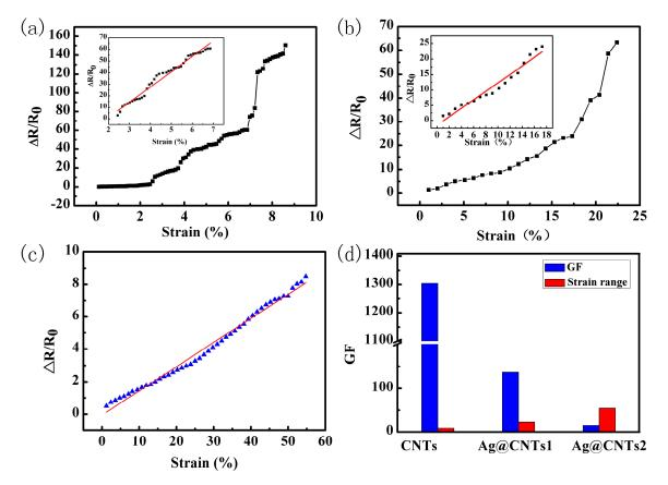
**Figure 6.** Relative resistance changes of the sensors with (**a**) CNTs, (**b**) Ag@CNTs1, and (**c**) Ag@CNTs2. (**d**) Relationships between Ag nanoparticle contents and as-prepared sensors' GFs and strain ranges.
