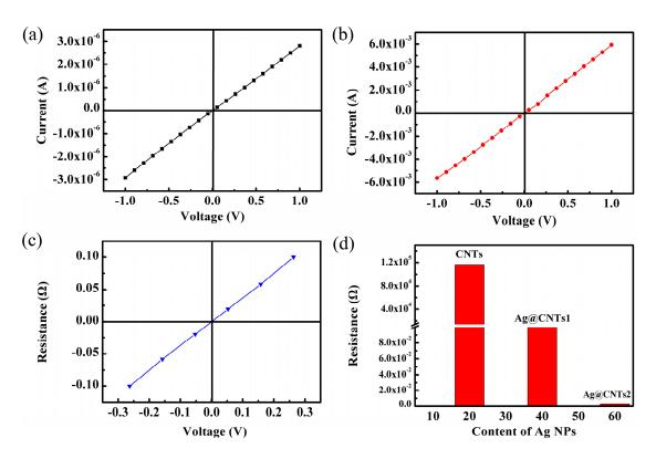
**Figure 5.** I-V curves of the sensors with (**a**) CNTs, (**b**) Ag@CNTs1, (**c**) Ag@CNTs2, and (**d**) the relationship between Ag nanoparticle contents and as-prepared sensors' resistivities.
