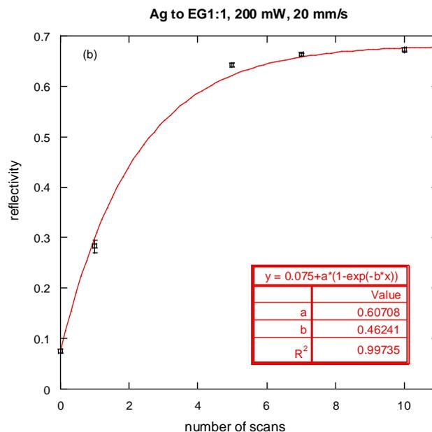
**Figure 7.** (a) Thickness of the silver film (b) reflectivity for 532 nm wavelength light *versus* number of laser scans (symbols: experimental data, lines: fitted curves).
