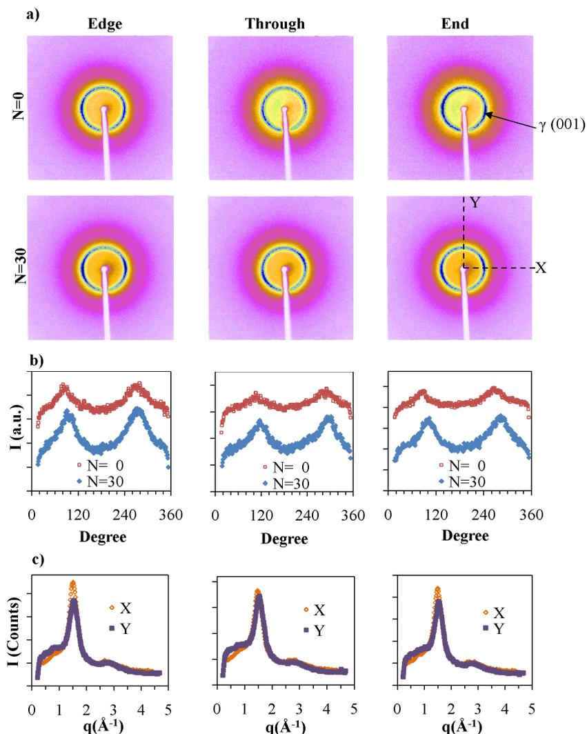
**Figure 8.** (a) Two-dimensional X-ray pattern of PA6 films at  $N = 0$  and  $N = 30$  from edge, through and end directions. The white regions in the middle of the images correspond to the shadow of the beam stopper; (b) The intensity along the  $\gamma$  crystalline ring marked in  $\gamma$  for the different directions; and (c) The cross sections of the  $N = 30$  along the  $X$  and  $Y$  directions.
