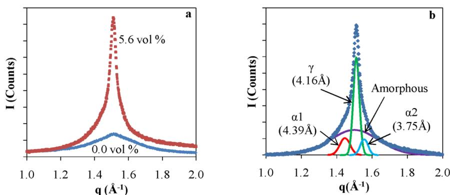
**Figure 5.** (a) Powder X-ray patterns of extruded PA6 with and without NPs at  $N = 0$ ; and (b) Peak deconvolution of X-ray data for 5.6 vol % nanocomposite.
