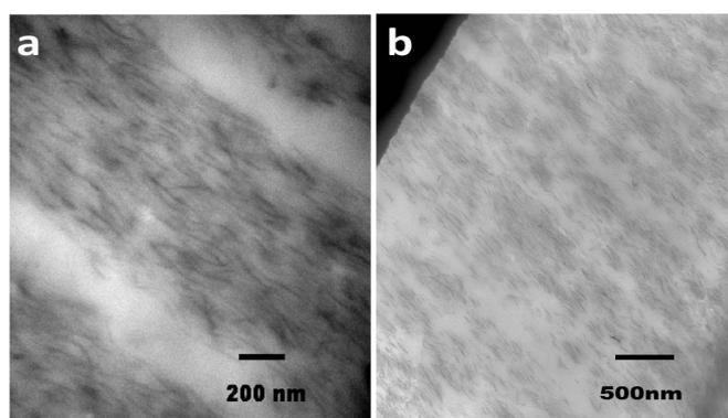
**Figure 1.** Transmission electron microscopy (TEM) image of (a) 2 vol % nanoparticles (NPs) montmorillonite nanocomposite formed by chaotic advection at  $N = 9$  [27]; and (b) 5.6 vol % at  $N = 7$ , extruded as 150 micron thick films. Dark regions correspond to the NP rich areas and light regions correspond to the matrix polymer.
