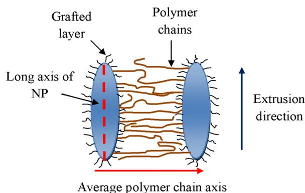
**Figure 10.** A schematic representation of the relative orientations of NPs and PA6 chains in nanocomposites.
