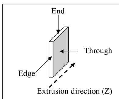
**Figure 3.** Directions of incident X-ray beams with respect to the extrusion direction.  $X$  and  $Y$  define the plane of the film and  $Z$  corresponds to the extrusion directions.
