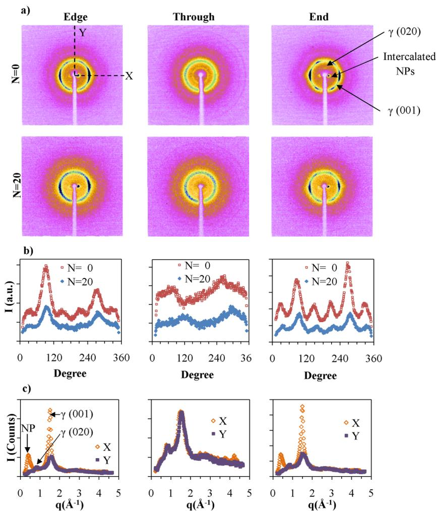
**Figure 9.** (a) Two dimensional X-ray patterns of PA6 with 5.6 vol % NP nanocomposite films at  $N = 0$  and  $N = 20$  from edge, through and end directions; (b) The intensity along the  $\gamma$  crystalline ring marked in  $\gamma$  for the different directions; and (c) The cross sections of the  $N = 0$  along  $X$  and  $Y$  directions.
