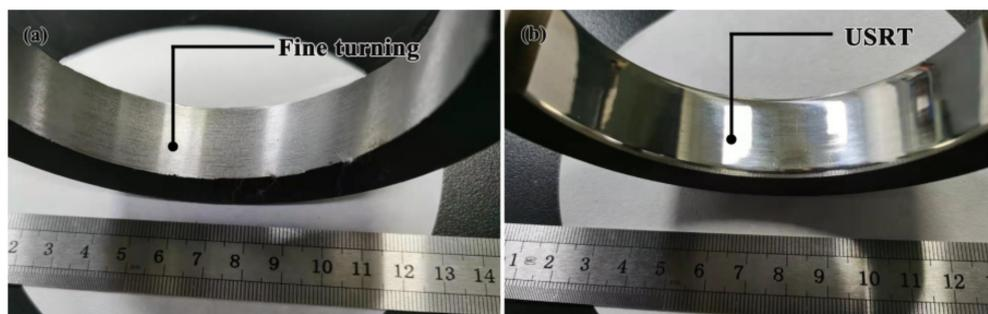
**Figure 2.** Comparison of the surface quality of AISI 304 stainless steel before (a) and after (b) the USRT processing.
