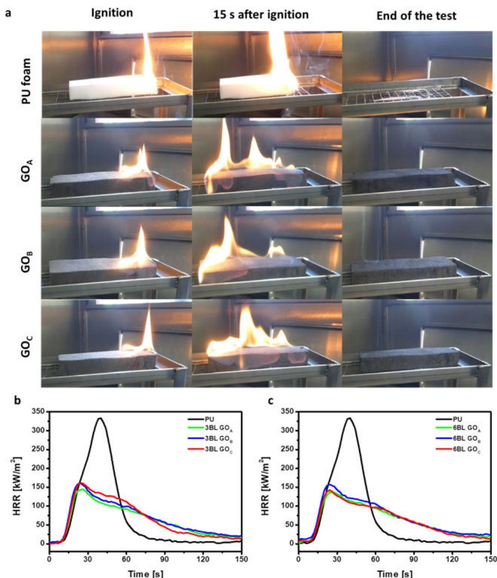
**Figure 5.** Flame retardant characterization: (a) Pictures of flammability test in horizontal configuration of untreated PU foam, 3BL CHIT/GO<sub>A</sub> treated PU foam, 3BL CHIT/GO<sub>B</sub> PU foam and 3BL CHIT/GO<sub>C</sub> PU foam. First column: right after ignition, second column: 15 s after ignition and third column: end of the test. (b) HRR vs time plots of 3BL samples. (c) HRR vs time plots of 6BL samples.
