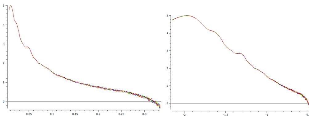
**Figure S4.** X-ray scattering curves of w/o  $\text{Co}^{\text{II}}@/\text{SiO}_2$  in logarithmic (**left**) and double logarithmic (**right**) scale. Different colors of curves are corresponded to 8 consistent experiments.
