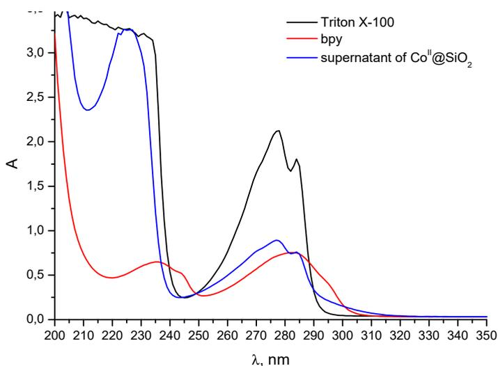
**Figure 1.** UV-vis spectra of supernatant diluted 300 times by ethanol after synthesis of w/o  $\text{Co}^{\text{II}}@\text{SiO}_2$  ( $\text{Co}^{\text{II}}(\text{bpy})_3$  as precursor) (**blue**) and ethanol solutions of bpy ( $C = 5 \times 10^{-5} \text{ mol} \cdot \text{L}^{-1}$ , **red**) and Triton X-100 ( $C = 0.9 \text{ g} \cdot \text{L}^{-1}$ , **black**).
