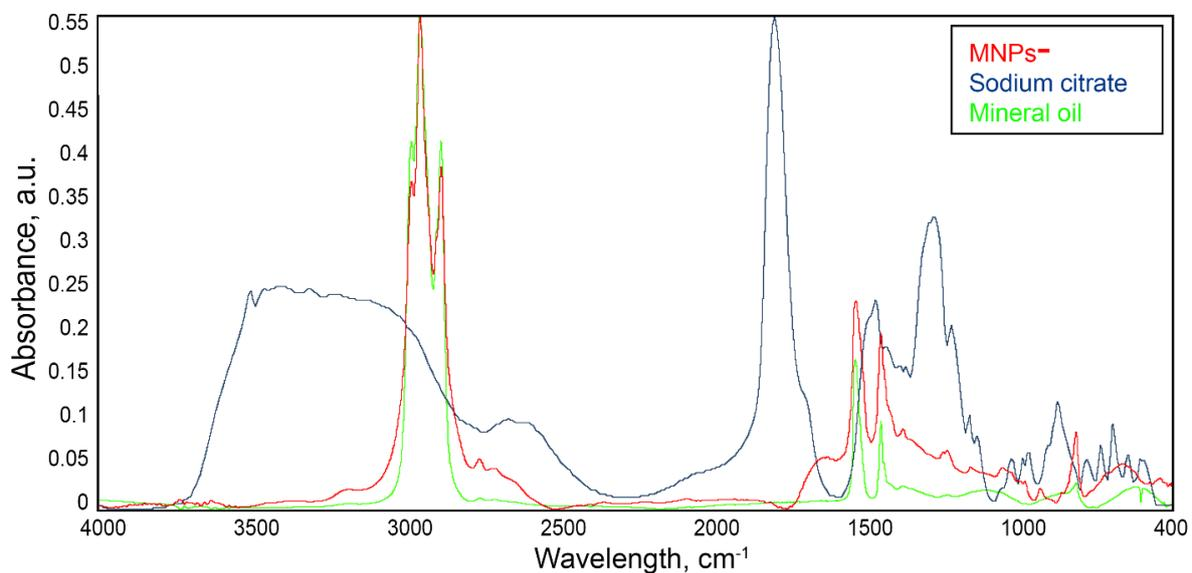
**Figure S3.** Fourier-transform infrared spectroscopy (FTIR) spectra of MNPs, sodium citrate, and the embedding medium (mineral oil).
