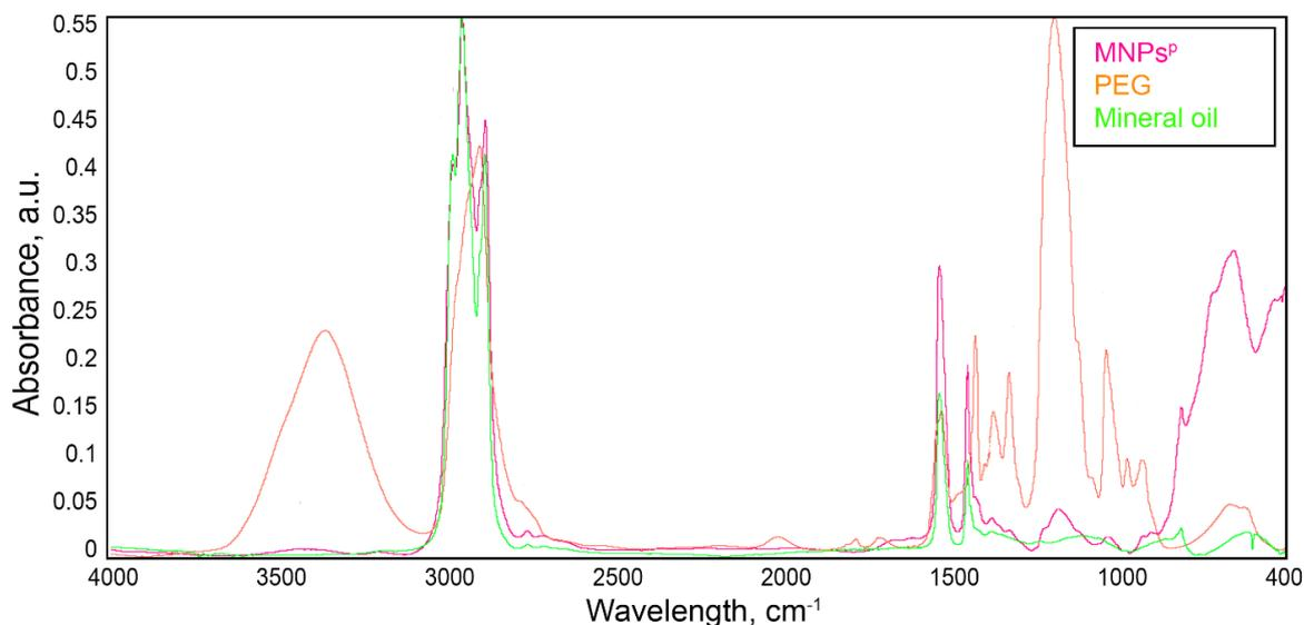
**Figure S4.** FTIR spectra of MNPs<sup>p</sup>, polyethylene glycol (PEG), and the embedding medium (mineral oil).
