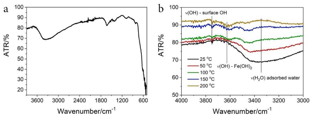
**Figure S2.** Attenuated total reflection infrared spectra (IR-ATR) of MNPs: (a) FTIR spectra of MNPs; and (b), water removal at elevated temperatures, reveals the presence of OH-groups on the surface of MNPs.
