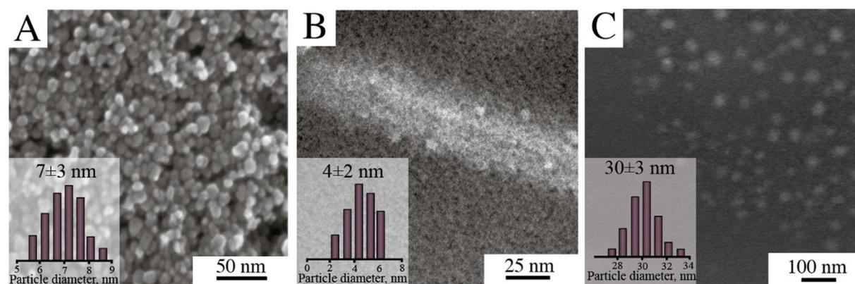
**Figure S1.** SEM images and particle size distribution of NPs: (A) magnetite nanoparticles (MNPs); (B) silica nanoparticles (SNPs); and (C) gold nanoparticles with average diameter 30 nm (GNP-30).
