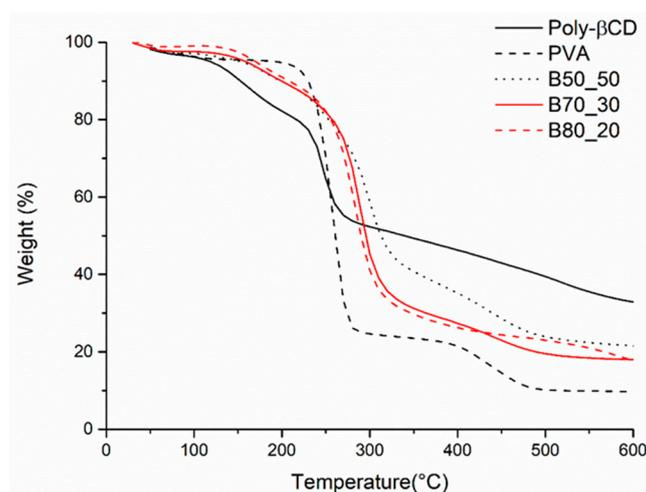
**Figure 3.** TGA curves of Poly- $\beta$ CD (red solid line), PVA (red dashed line), B50\_50 (black solid line), B70\_30 (black dashed line), and B80\_20 (black dotted line).
