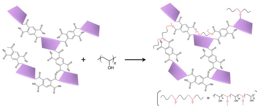
**Figure 2.** Scheme of the cross-linking reactions between Poly- $\beta$ CD and PVA during the curing treatment.
