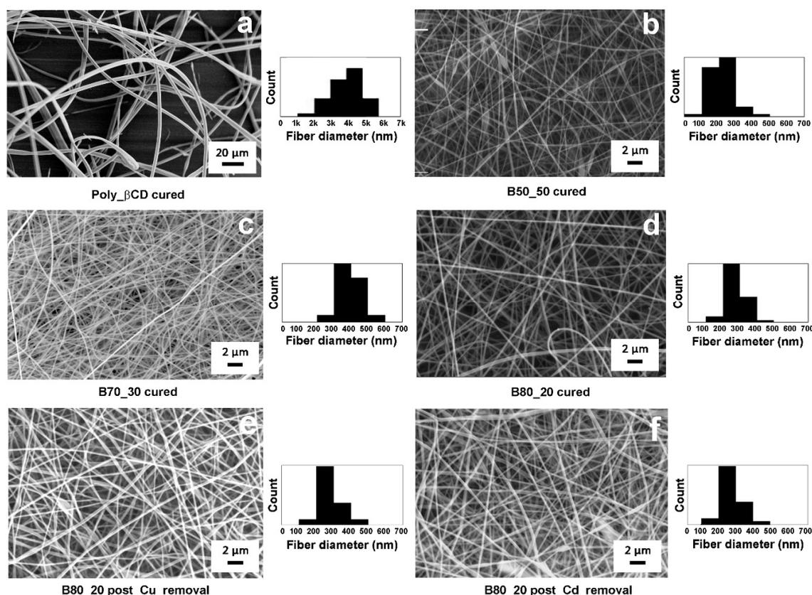
**Figure 7.** SEM micrographs of cured fibers and histograms showing the fiber diameter distribution: Poly-βCD (a), B50\_50 (b), B70\_30 (c), B80\_20 (d), B80\_20 after adsorption and desorption of copper (e) and cadmium (f).
