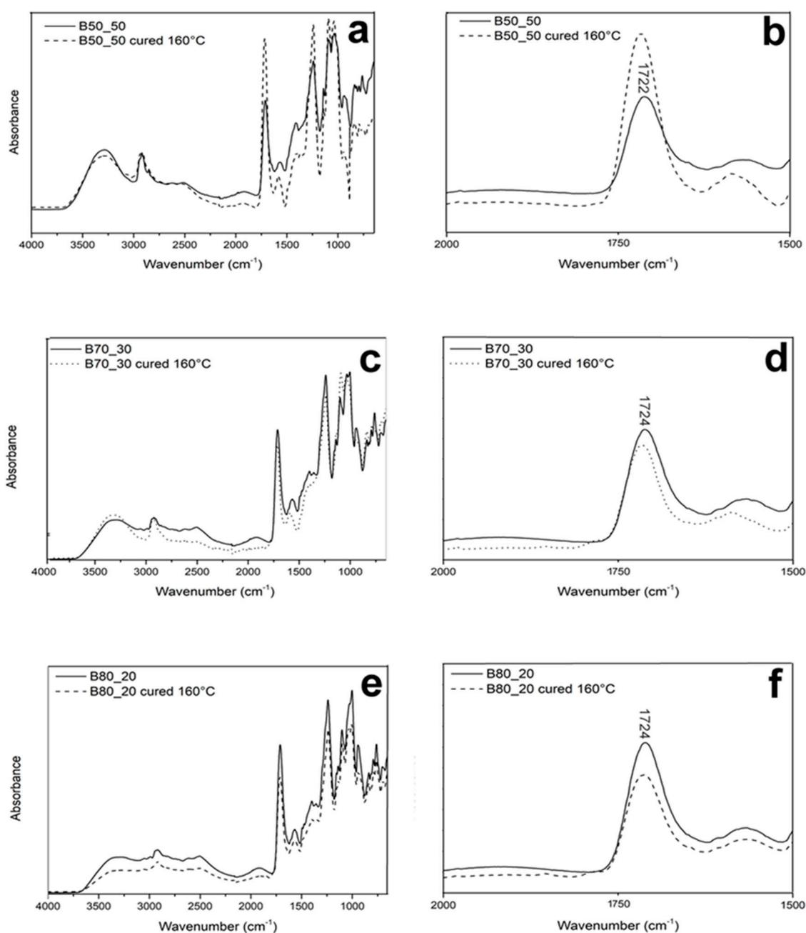
**Figure 5.** Full attenuated total reflectance mode (ATR-FTIR) spectra of as-spun and cured fibers: B50\_50 (a), B70\_30 (c), and B80\_20 (e). Magnification of the C=O stretching: B50\_50 (b), B70\_30 (d), and B80\_20 (f).
