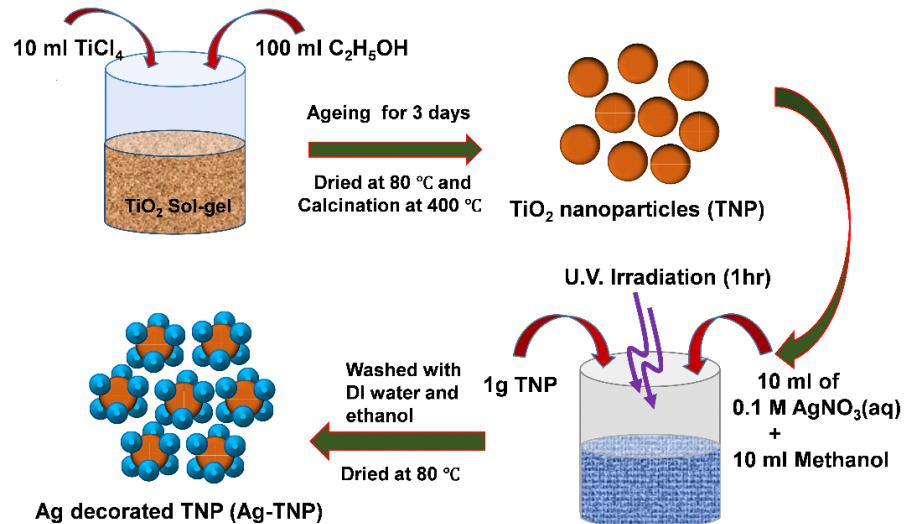
**Figure S1** Detailed schematic illustrates of synthesis route of Ag-TNP.
