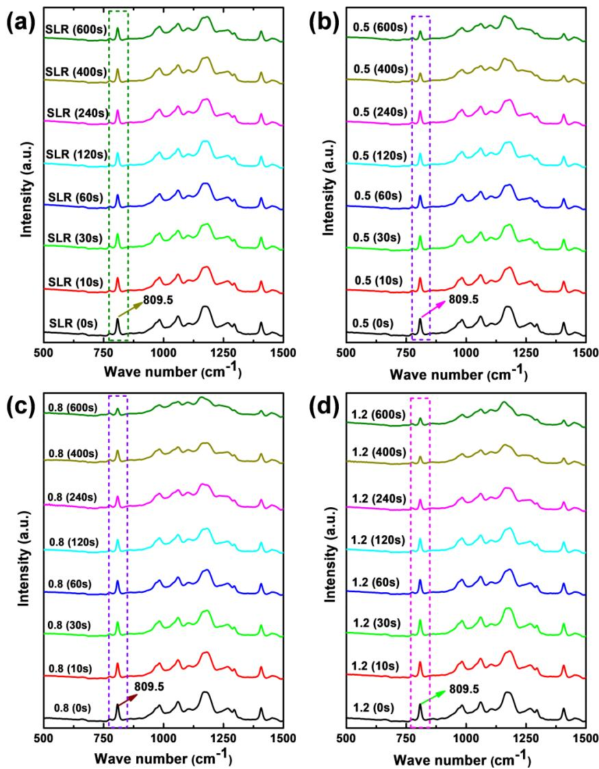
**Figure S5** A real time FTIR analysis of photopolymerization of (a) neat SLR, (b) SLR/Ag-TNP-0.5, (c) SLR/Ag-TNP-0.8 and (d) SLR/Ag-TNP-1.2, nanocomposites in different periods of time intervals starting from 0 s to 600 s under the UV irradiation power of 32 mW/cm<sup>2</sup>.
