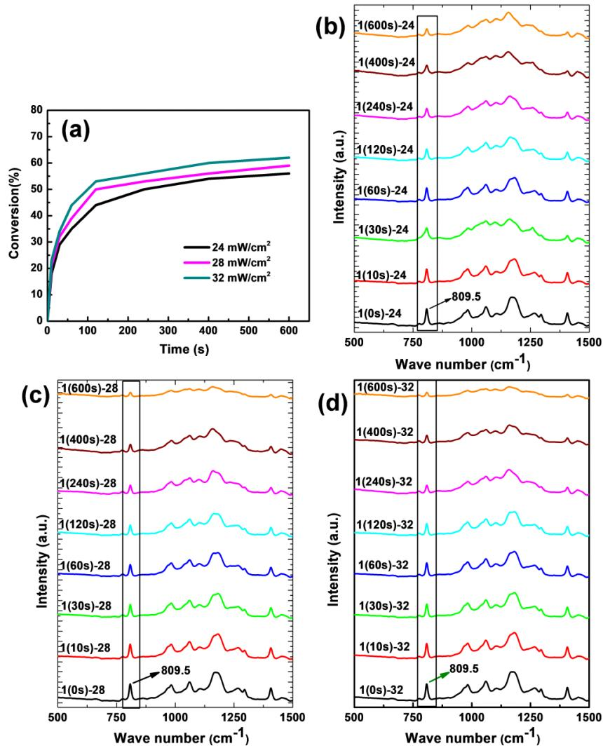
**Figure S6** (a) Percentage conversion graph of SLR/Ag-TNP-1 nanocomposite in different power densities of UV-irradiation monitored by RT-FTIR. (b), (c) and (d) are real time FTIR analysis of photopolymerization of SLR/Ag-TNP-1 nanocomposites in different periods of time intervals starting from 0 s to 600 s under UV irradiation power densities of 24mW/cm<sup>2</sup>, 28mW/cm<sup>2</sup> and 32mW/cm<sup>2</sup> respectively.
