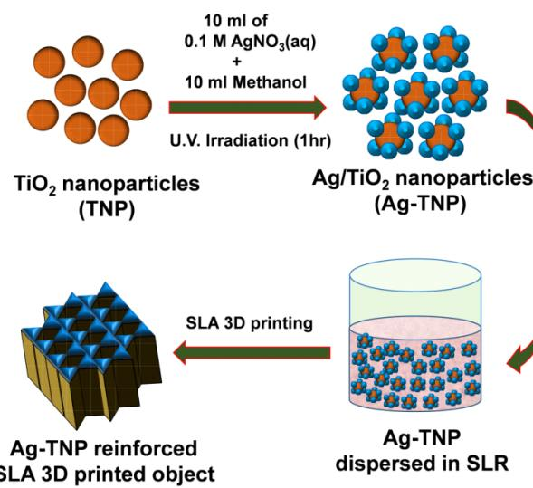
**Figure S2** The step by step detailed preparation route of SLR/Ag-TNP nanocomposites.
