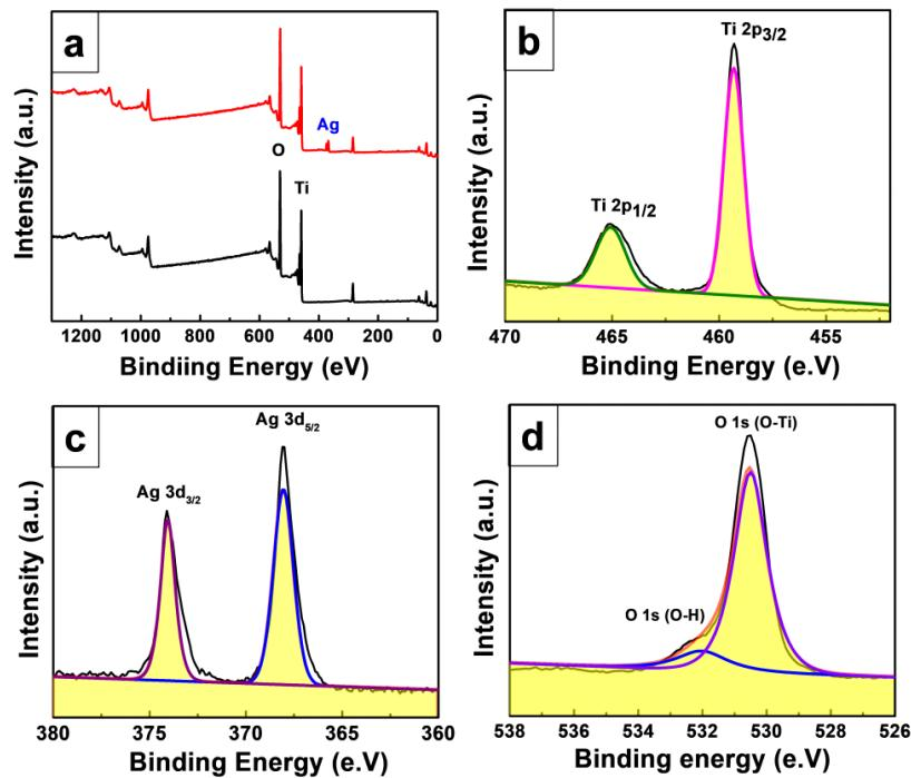
**Figure S4** XPS spectrum analysis of as-prepared  $\text{TiO}_2$ , and Ag/TNP (a) survey spectrum (black spectrum represents  $\text{TiO}_2$  and red spectrum represents Ag-TNP), (b) Deconvoluted XPS spectra of Ti, and (c) Deconvoluted XPS spectra of Ag, (d) Deconvoluted XPS spectra of O.
