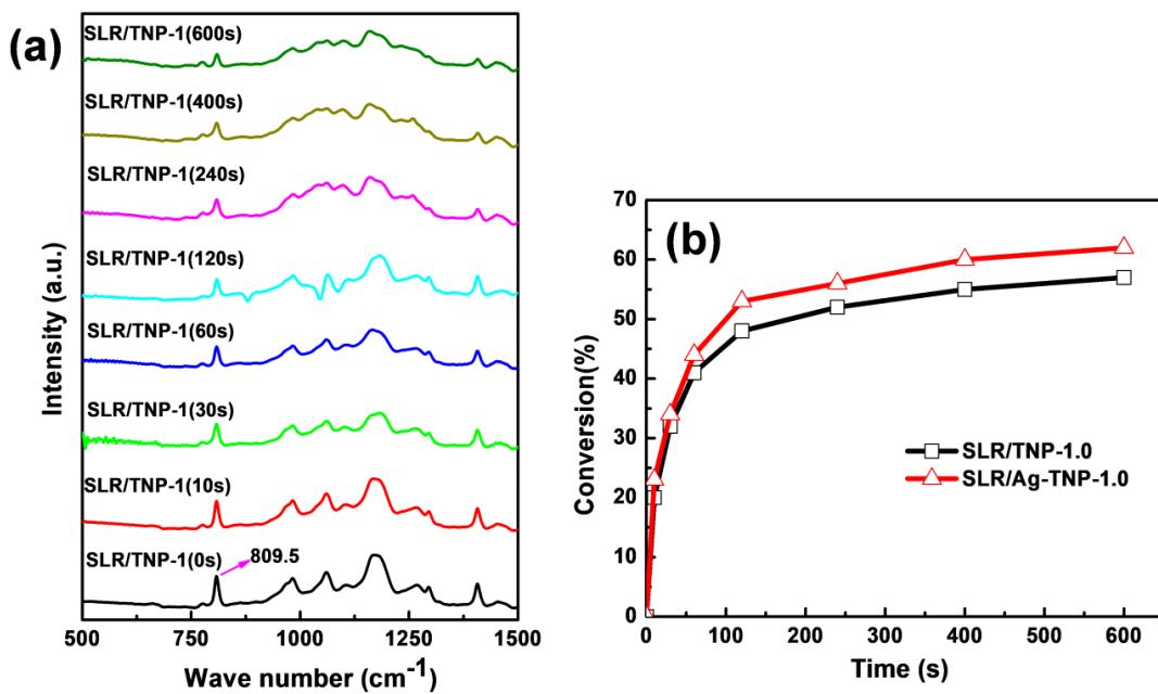
**Figure S7** (a) Real time FTIR analysis of SLR/TNP-1 nanocomposite and (b) Percentage conversion graph of photopolymerization of SLR/TNP-1 nanocomposite (black line) and SLR/Ag-TNP-1 (red line) nanocomposite, under the UV irradiation power of 32mW/cm<sup>2</sup> in different periods of time intervals starting from 0 s to 600 s.
