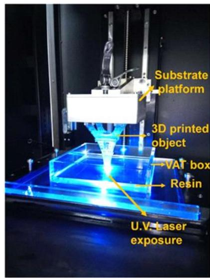
**Figure S3** The digital image of the SLA 3D printing device, which was utilized for this research work.
