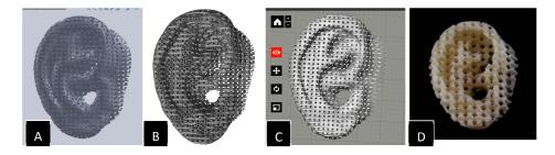
**Figure 1.** Sequential steps involved in a 3D printing process. (**A**) Designed 3D computer aided design (CAD) model; (**B**) Stereolithography (STL) file of the model; (**C**) Slicing or 3D printing software; (**D**) 3D printed object.
