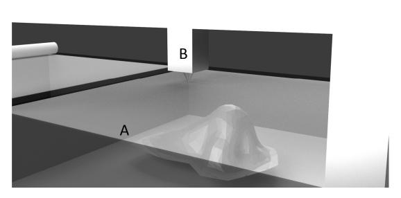
Figure 4. Inkjet 3D printing. (A) Powdered bed; (B) Binding liquid spraying nozzle.
