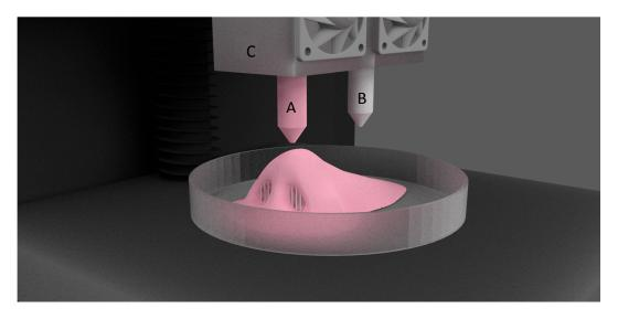
Figure 2. Dual head FDM 3D printer. (A) Building material; (B) Supporting material; (C) Print heads.
