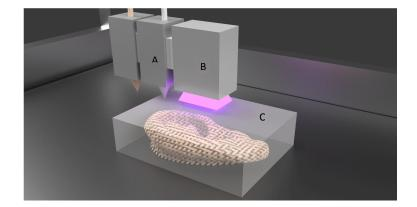
Figure 5. Polyjet 3D printer. (A) Nozzle spraying photopolymer; (B) UV source; (C) Supporting material.
