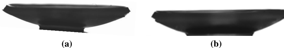
Figure 2. Femtosecond laser-assisted tophat cuts of the BDDGE cross-linked hydrogels that were cross-linked (a) at pH 11; and (b) at pH 5, with subsequent cross-linking with EDC/NHS.
