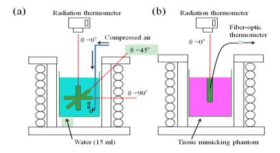
**Figure 2.** Complete experimental setup for measuring the heat transfer behavior of the tissue-mimicking phantom subjected to the insertion of the Ti-coated carbon steel rod in the high-frequency induction field of 1.69 kA/m at 300 kHz.
