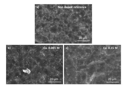
**Figure 5.** SEM micrographs of an undoped CaP-coated sample after 1 min of electrodeposition (**a**), after its doping by an ion exchange post-treatment using a copper ion solution of 0.001 M (**b**) or of 0.15 M (**c**).
