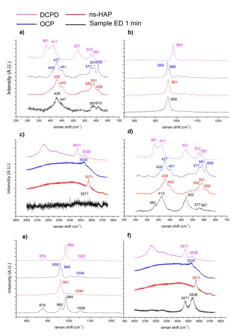
**Figure 3.** Raman spectra of DCPD, OCP, and ns-HAP reference powders and CaP-coated sample after 1 min of electrodeposition: (**a**–**c**) on the layer of nano-needles, and (**d**–**f**) on micro-platelet crystals.
