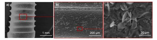
**Figure 10.** SEM micrographs showing an undoped CaP-coated titanium dental implant after 1 min of electrodeposition at three magnifications (from low (**a**) to higher magnification (**b**) and then (**c**). The focus area corresponding to (**b**,**c**) is indicated by the red rectangle on (**a**,**b**), respectively).
