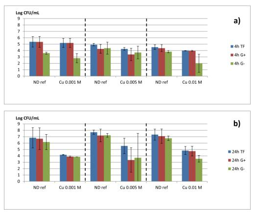
**Figure 8.** CFU/mL (mean  $\pm$  SD) of Gram-positive (G+) and negative (G-) strains and total flora (TF) on non-doped CaP-coated samples (ND ref) and on Cu-doped CaP-coated samples (after exchange in 0.001, 0.005, or 0.01 M copper ion solutions) after 4 h (**a**) and 24 h (**b**) from inoculation.
