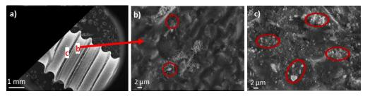
**Figure 11.** SEM micrographs of an undoped 1 min-CaP-coated titanium dental implant after the screwing and unscrewing test in an artificial jawbone: (a) General view and indication of the location of b and c focus area; (b) At the thread bottom; and (c) At the thread top of the dental implant. The red circles show that some bright particles corresponding to debris of the artificial jawbone remained stuck to the implant.
