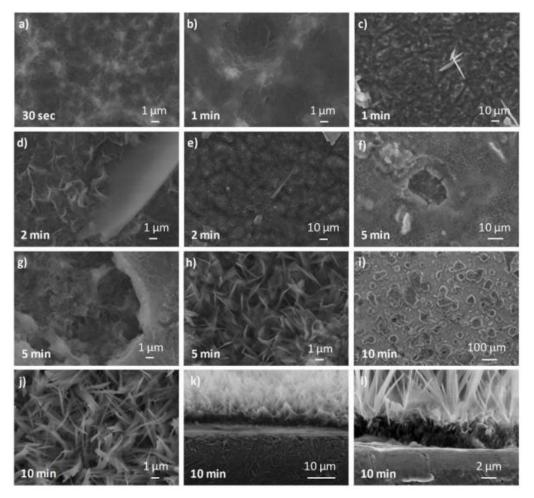
**Figure 1.** SEM micrographs of calcium phosphate coatings obtained after an electrodeposition time of: (a) 30 s; (b,c) 1 min; (d,e) 2 min; (f–h) 5 min; and (i–l) 10 min; (k,l) Cross-section of the substrate-coating interface for the 10 min electrodeposited sample.
