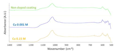
**Figure 6.** FTIR-ATR spectra of copper-doped CaP-coated samples using 0.001 M and 0.15 M copper solutions for ion exchange post-treatment in comparison with an undoped CaP-coated sample (obtained after 1 min of electrodeposition).
