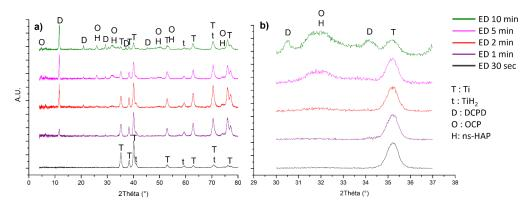
**Figure 2.** XRD patterns of the calcium-phosphate-coated samples obtained after different electrodeposition times (30 s, 1, 2, 5, and 10 min): (a) from  $2\theta = 4^{\circ}$  to  $80^{\circ}$ , and (b) from  $2\theta = 29^{\circ}$  to  $38^{\circ}$ .
