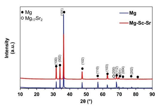
**Figure 1.** XRD patterns of the Mg and Mg-Sc-Sr alloy showing  $\alpha$ -Mg phase for Mg sample and  $\alpha$ -Mg and Mg<sub>17</sub>Sr<sub>2</sub> intermetallic phase for Mg-Sc-Sr alloy.
