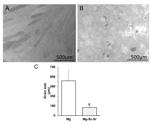
**Figure 3.** Metallography images: (**A**) Mg, (**B**) Mg-Sc-Sr, (**C**) average grain sizes of the Mg and Mg-Sc-Sr discs. In comparing the Mg-Sc-Sr grain size to the Mg grain size, a significant reduction in grain size for Mg-Sc-Sr was observed. Significant differences: a: p < 0.05 Mg-Sc-Sr vs. Mg.
