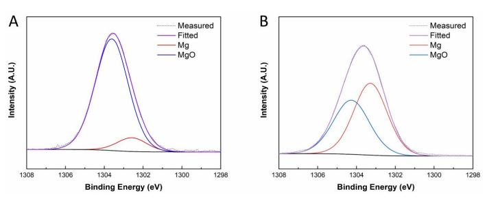
**Figure 2.** XPS spectra: **(A)** Mg 1s for Mg sample, **(B)** Mg 1s for Mg-Sc-Sr sample. We observed a lower oxide proportion relative to the Mg-Sc-Sr sample's metallic state.
