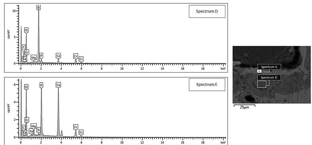
**Figure 6.** EDS compositional analysis: bi-layered reaction layer formed on the surface of a robocast scaffold subjected to static soaking in SBF inside a traditional incubator (area D = silica gel, area E = hydroxyapatite).
