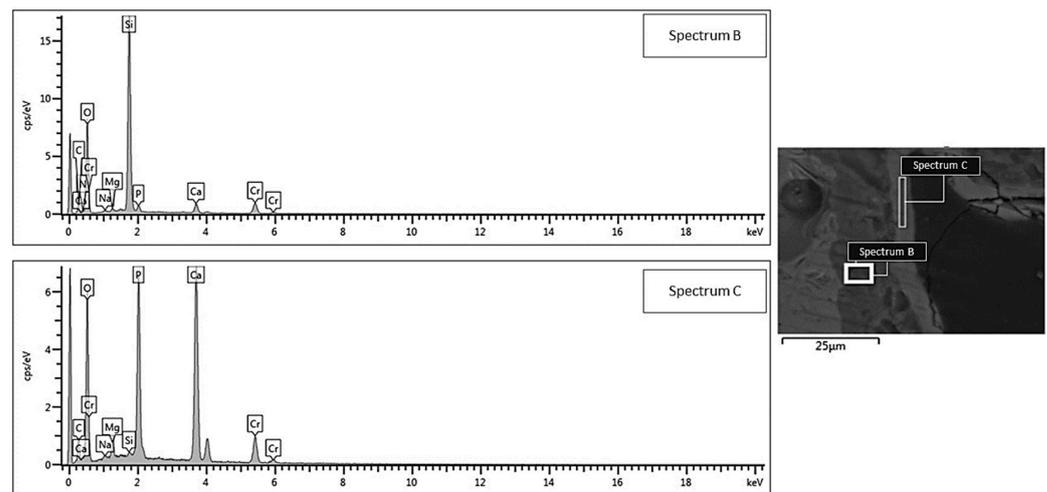
**Figure 5.** EDS compositional analysis: bi-layered reaction layer formed on the surface of a robocast scaffold subjected to mild shaking in SBF inside an orbital shaker incubator (area B = silica gel, area C = hydroxyapatite).
