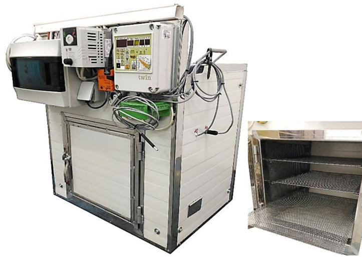
**Figure 1.** Laboratory-scale convective dryer and three-perforated tray drying chamber.
