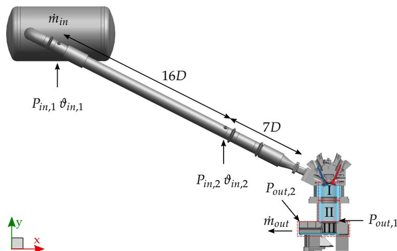
**Figure 2.** Flow bench and intake system overview. The inner diameter of the intake pipes  $D$  is 56.3 mm. Experimental sections include the standard engine- (I), the Flow bench- (II) and the Outlet duct optical access (III).
