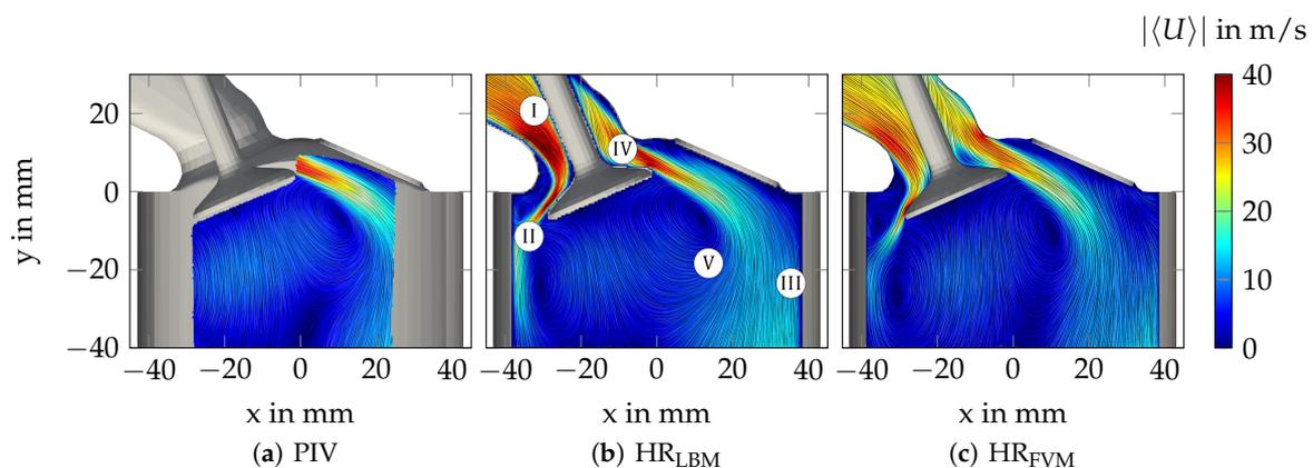
**Figure 6.** Line integral convolution visualization of the averaged velocity field with local characteristic flow patterns (I-V) of the PIV measurements (a), along with the OpenLB (b) and OpenFOAM (c) numerical results.
