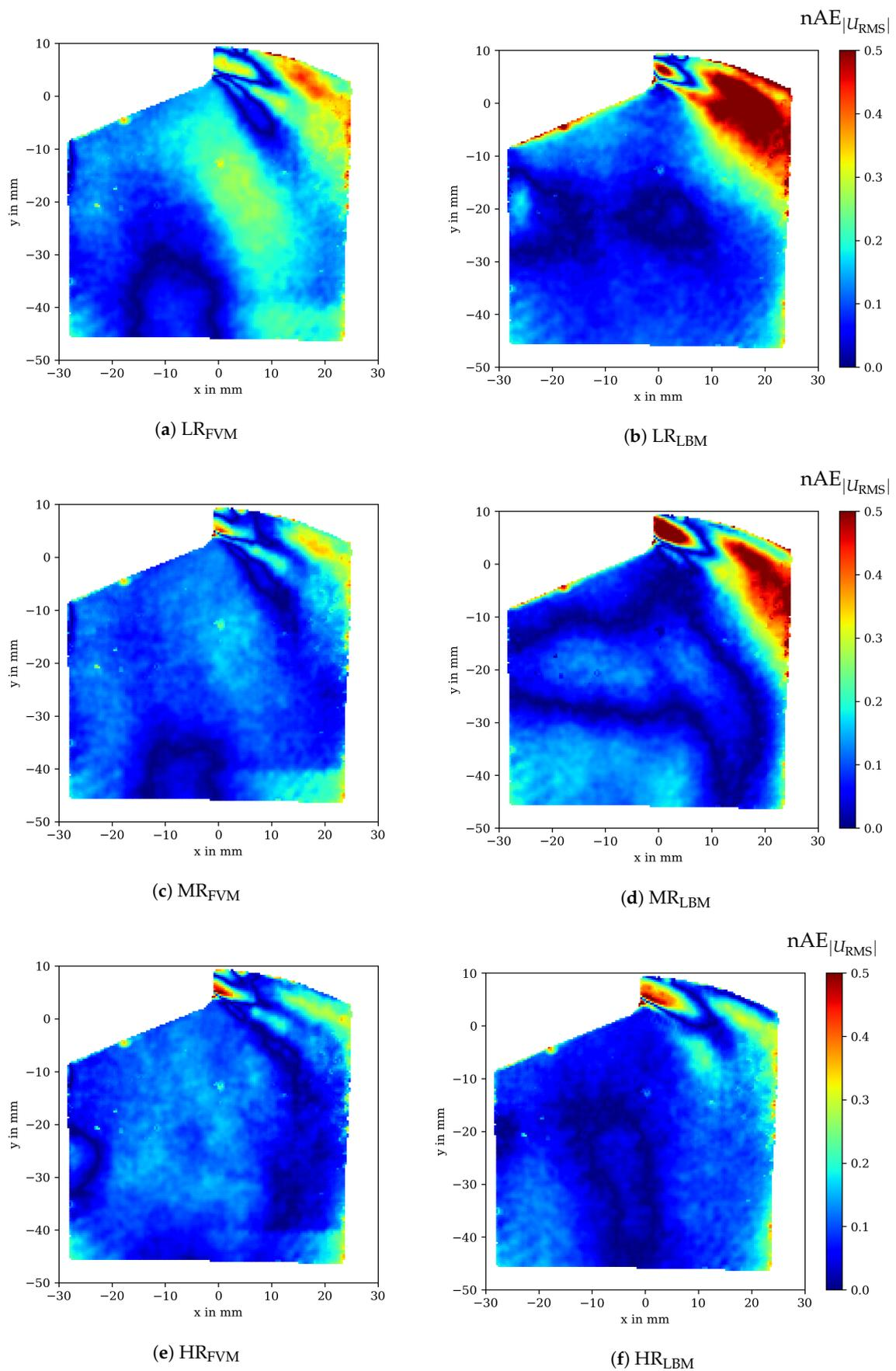
**Figure 11.** Normalized absolute error (nAE) map representation of the RMS velocity  $nAE_{|U_{RMS}|}$  for in-cylinder flow against PIV data for OpenFOAM (left) and OpenLB (right) at different grid resolutions.
