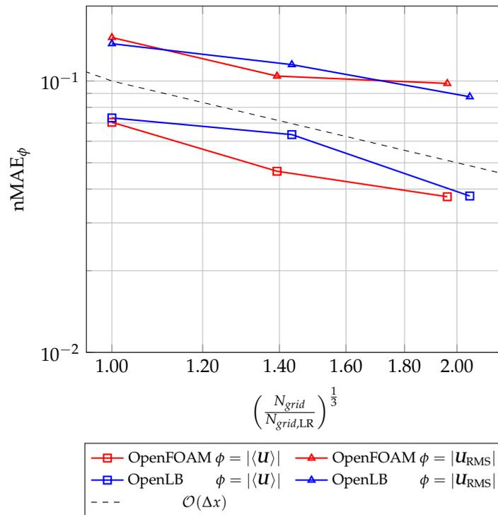
**Figure 12.** Normalized mean absolute error of the time-averaged velocity  $nMAE_{|\langle \mathbf{U} \rangle|}$  and the RMS velocity  $nMAE_{|\mathbf{U}_{RMS}|}$  for three different grids: low resolution (LR), median resolution (MR) and high resolution (HR). The number of cells are normalized by the coarse grid LR.
