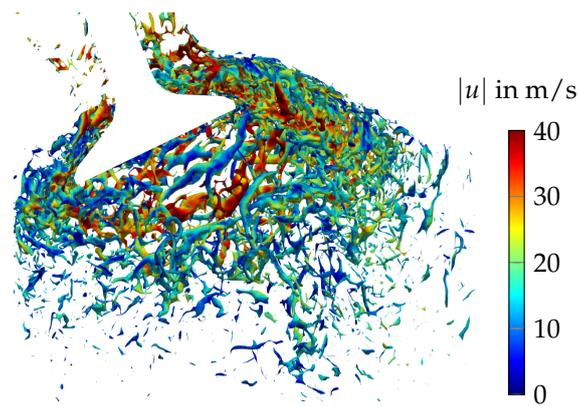
**Figure 7.** Turbulent structures as smoothed iso-surfaces of Q-criterion with  $Q = 7 \times 10^{-7}$  and magnitude of velocity from HR<sub>LBM</sub>.
