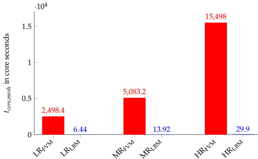
**Figure 13.** Meshing runtime  $t_{core,mesh}$  comparison between OpenFOAM and OpenLB for the three grid configurations: LR, MR and HR.
