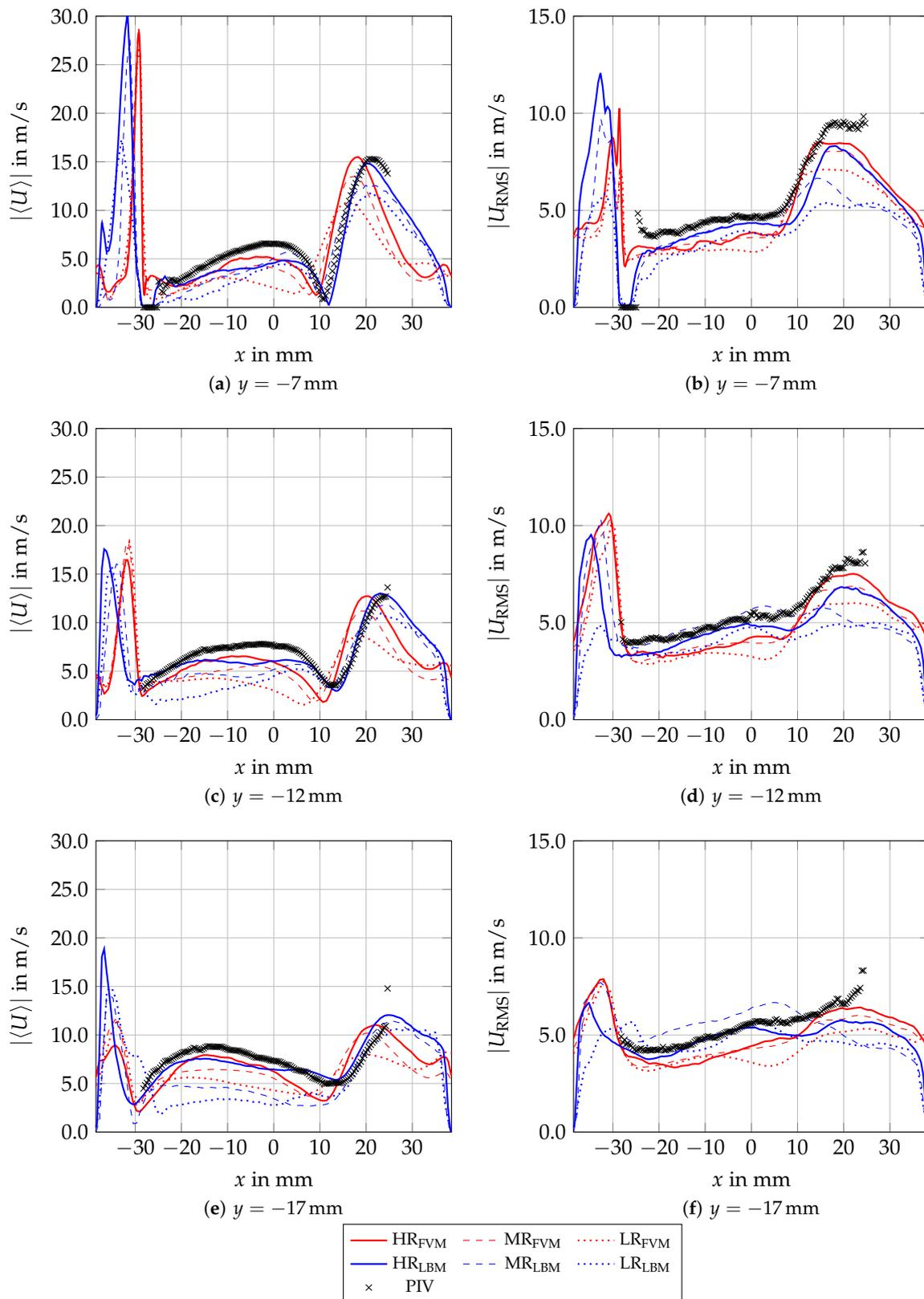
**Figure 9.** Magnitude of the two dimensional time-averaged velocity  $|\langle U \rangle|$  and root mean square (RMS) velocity  $|U_{RMS}|$  at  $y = -7\text{ mm}$ ,  $y = -12\text{ mm}$  and  $y = -17\text{ mm}$  in low, medium and high resolution grids for Lattice Boltzmann Method (LBM) and finite volume method (FVM) in comparison with PIV data.
