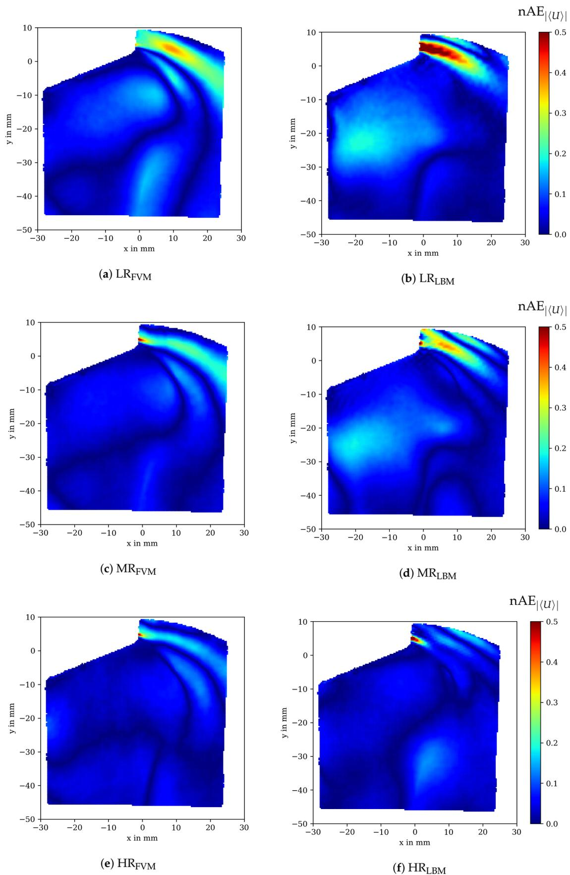
**Figure 10.** Normalized absolute error (nAE) map representation of the time-averaged velocity  $nAE_{|\langle U \rangle|}$  for in-cylinder flow against PIV data for OpenFOAM (left) and OpenLB (right) at different grid resolutions.
