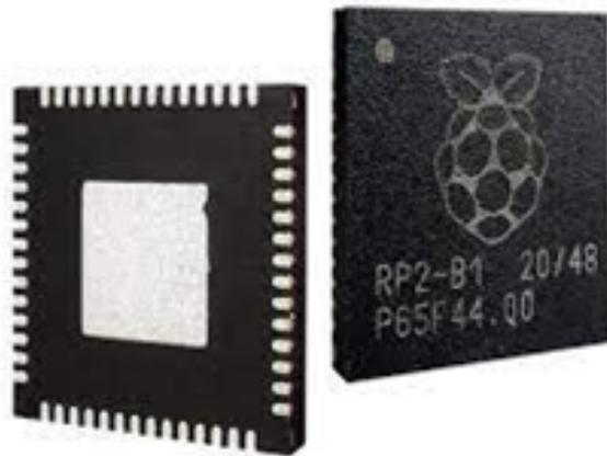
**Figure 18.** The Pi Pico processor RP2040.
