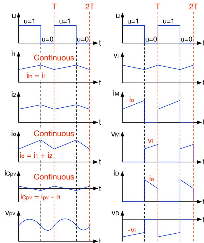
Figure 4. Waveforms of the PV system based on the CIOC buck converter.
