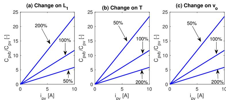
Figure 6. Input capacitor comparison between both buck converters.
