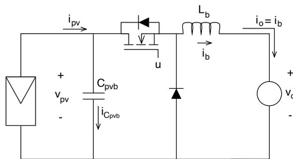
Figure 5. PV system based on the classical buck converter
