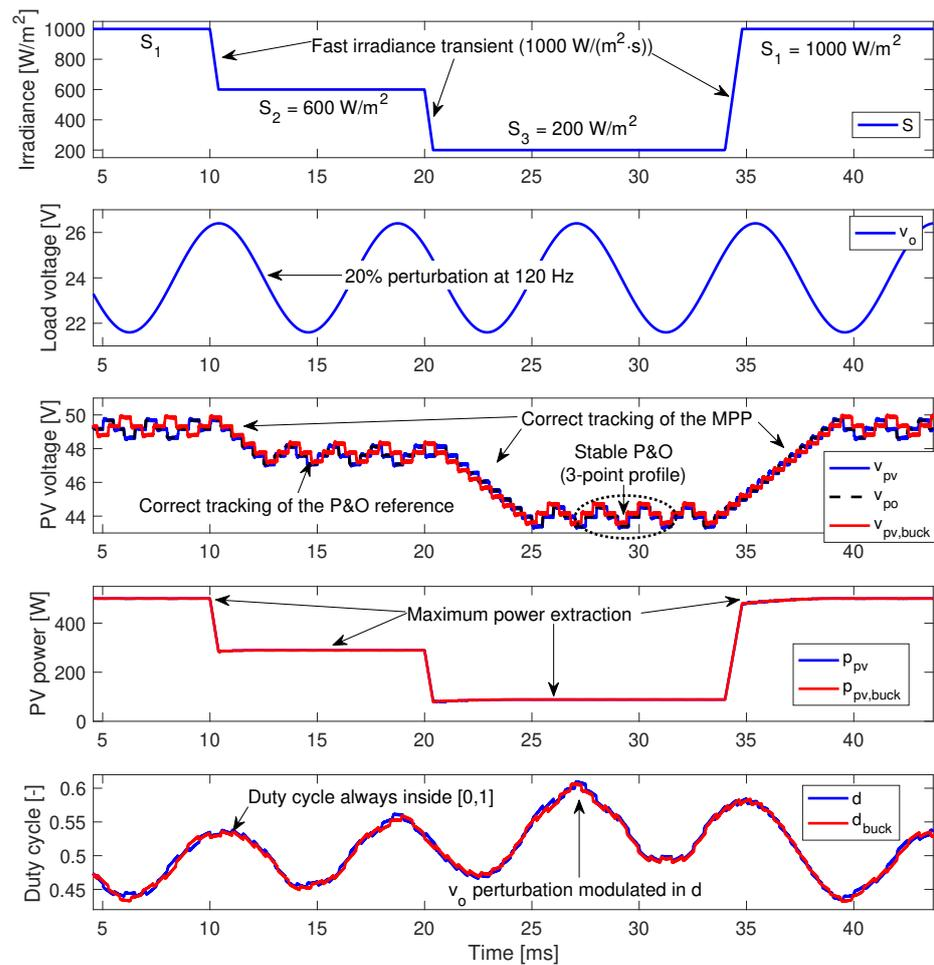
**Figure 17.** Maximum power point tracking using the CIOC converter with SMC and the classical buck converter with SMC.
