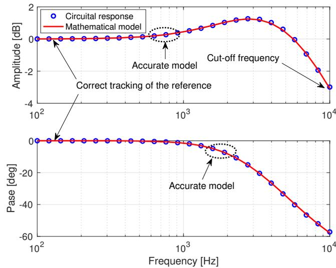
Figure 13. Frequency response of the PV system in closed loop.
