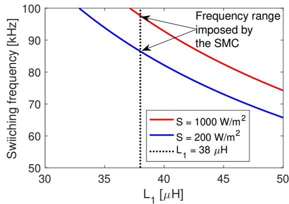
Figure 9. Design of the inductors in the CIOC converter.
