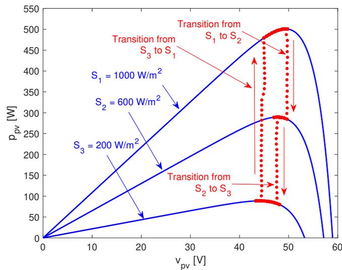
**Figure 18.** Maximum power point tracking trajectories.
