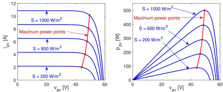
**Figure 8.** Electrical characteristics of the SP500M6-96 PV panel.
