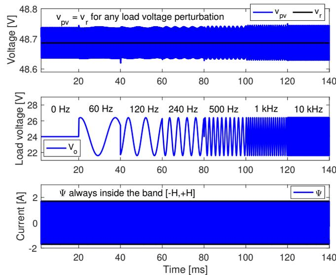
Figure 16. Performance of the PV system to different perturbations in the load voltage.
