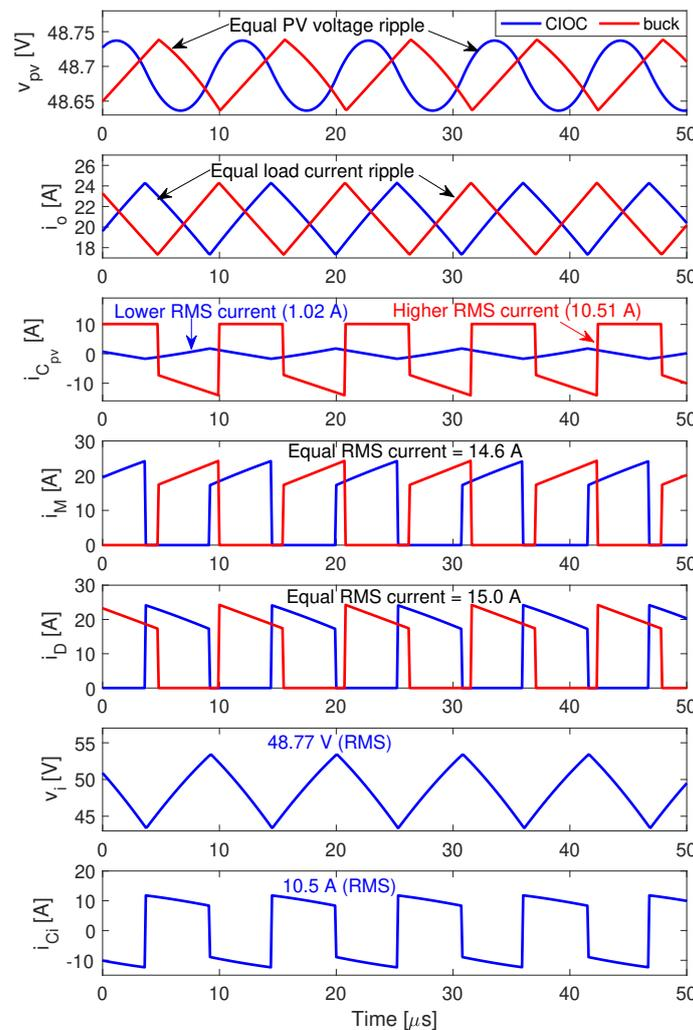
**Figure 12.** Performance comparison of PV systems based on both CIOC and classical buck converters.
