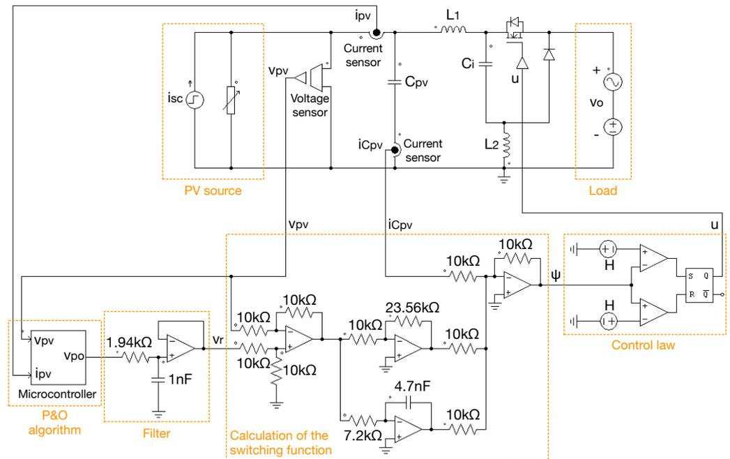
Figure 11. Circuitual implementation of the PV system based on the CIOC converter and SMC.
