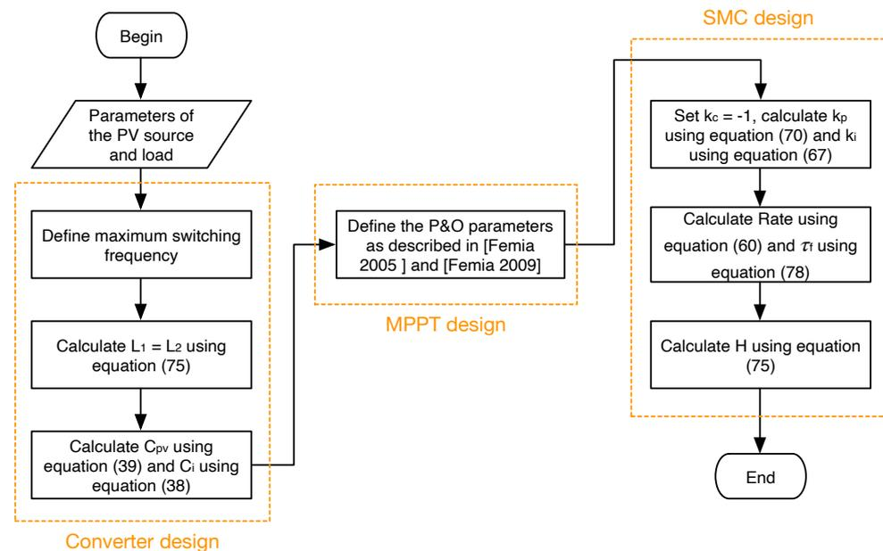
**Figure 10.** Flowchart of the proposed design process, where the P&O parameters are defined following [46,47].
