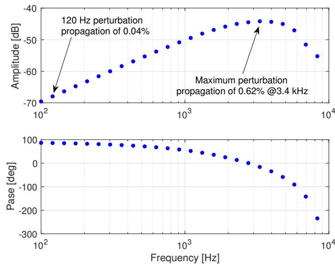
Figure 14. Perturbations mitigation in the closed-loop circuit.
