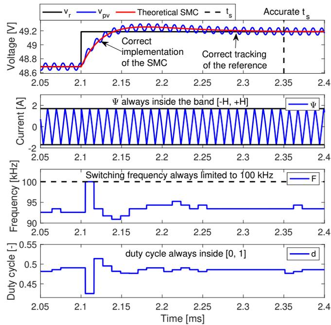
Figure 15. Performance of the PV system to changes on the reference value.
