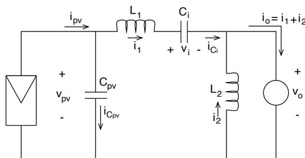
Figure 3. Topology 0 of the PV system based on the CIOC buck converter.
