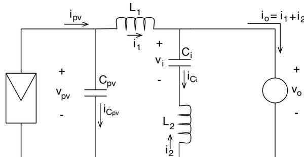
Figure 2. Topology 1 of the PV system based on the CIOC buck converter.
