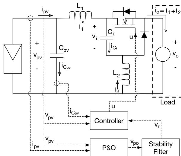
Figure 1. PV system based on the CIOC buck converter.
