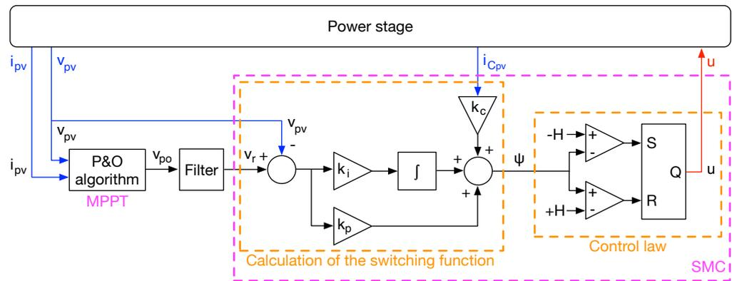
Figure 7. Block diagram of the proposed SMC (measured signals: blue lines; control signal: red line).
