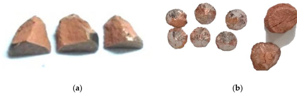
**Figure 11.** The remaining fragmentation of the actual ballistic testing (a) AMMO 1; (b) AMMO 2.
