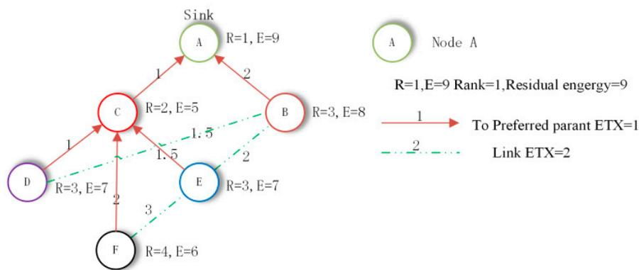
Figure 1. Topological structure based on ETX.
