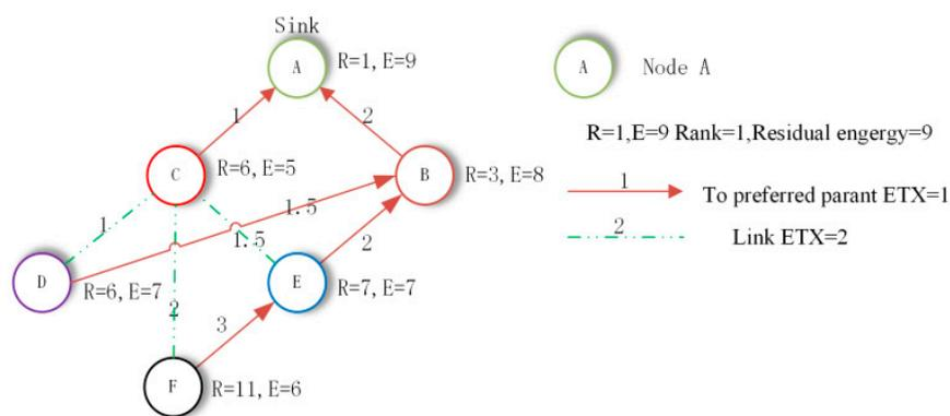
Figure 2. Network topology constructed according to the residual energy.
