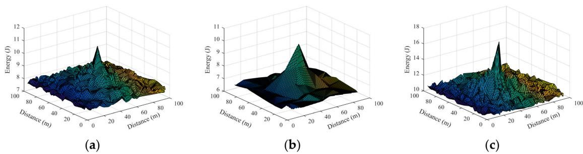
**Figure 7.** Residual energy distribution (cache size 30). (a) For original RPL; (b) For Algorithm 2; (c) For Algorithm 4.
