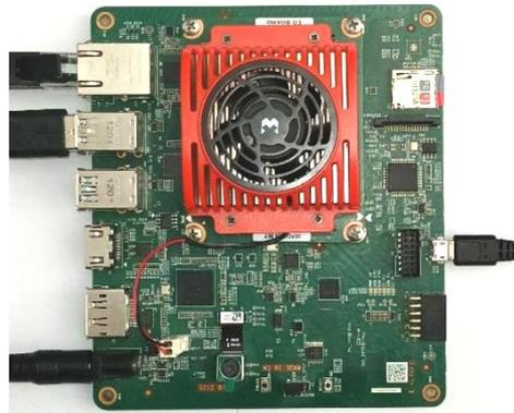
**Figure 5.** Xilinx KV260 FPGA hardware platform.
