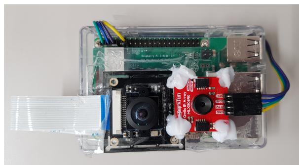
**Figure 2.** An image of the system built to collect the sensor frames and the camera images.
