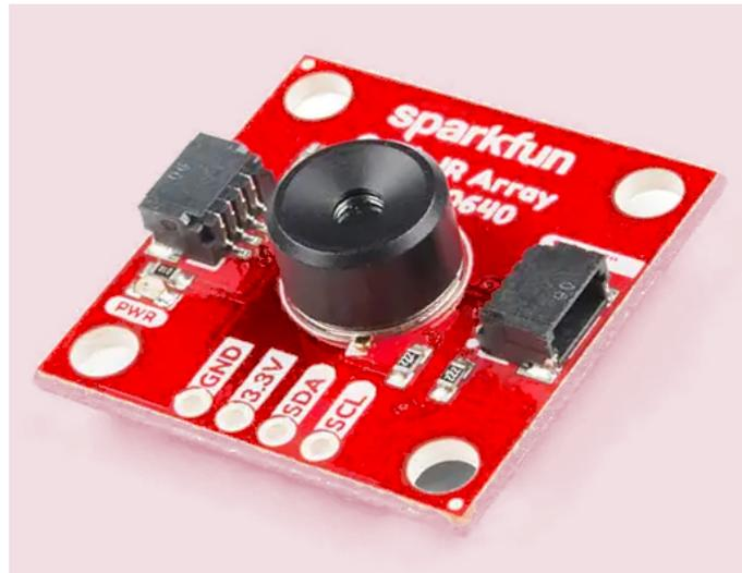
**Figure 1.** The IR array sensor used for our experiments.
