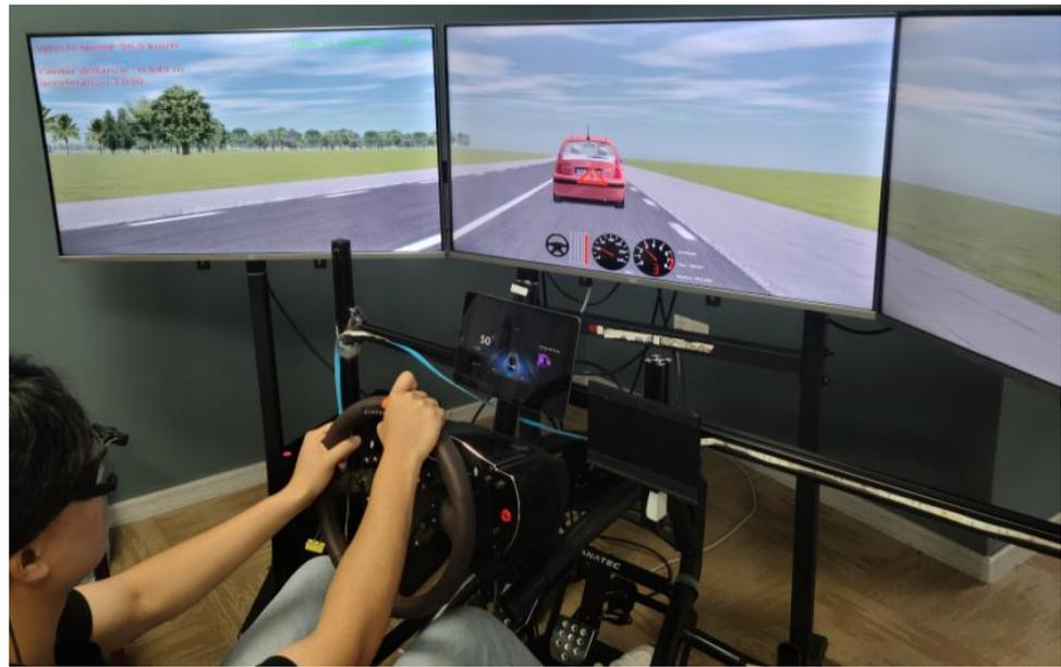
**Figure 2.** The open-cab driving simulator.
