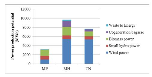
Figure 1. Source-wise renewable power production potential in the three states [19].
