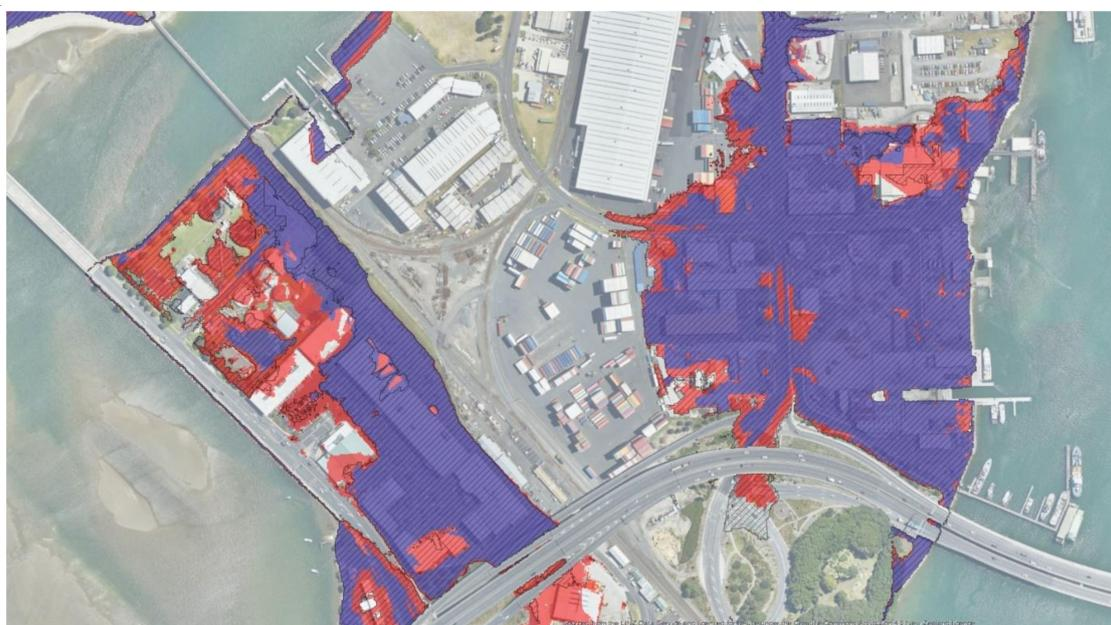
**Figure 6.** Comparison of model types for 1% AEP coastal flooding + 0.4 m RSLR, at a port storage facility in Tauranga Harbour. Red = dynamic, purple = static-planar, hashed = static-inclined.
