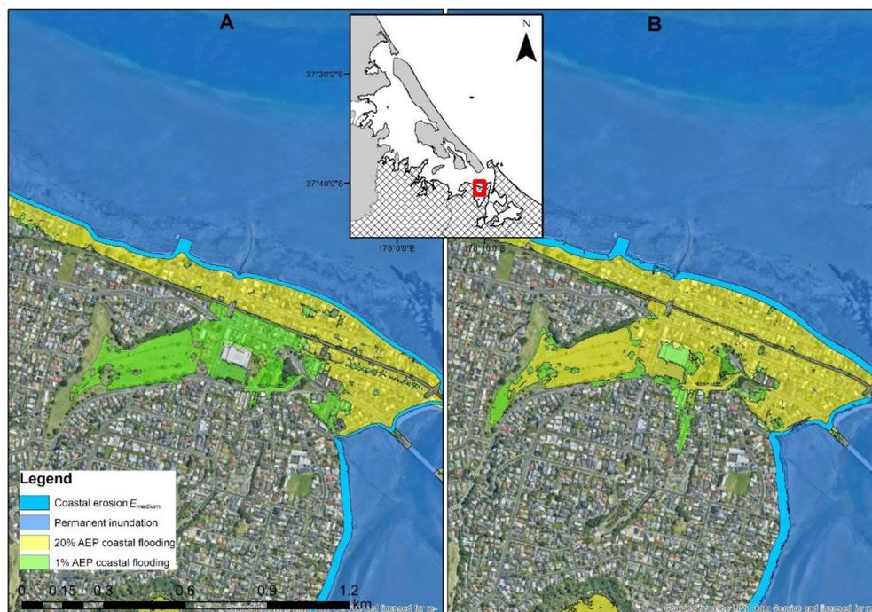
**Figure 7.** Comparison of hazard exposure extent for an area within Tauranga Harbour: (A) RSLR = 0.4 m, (B) RSLR = 0.6 m.
