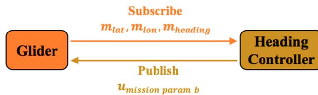
**Figure 18.** Exchange of data between the main vehicle control system and the heading controller when the glider changed its heading based on detection of a plume from a fluorometer measurement.
