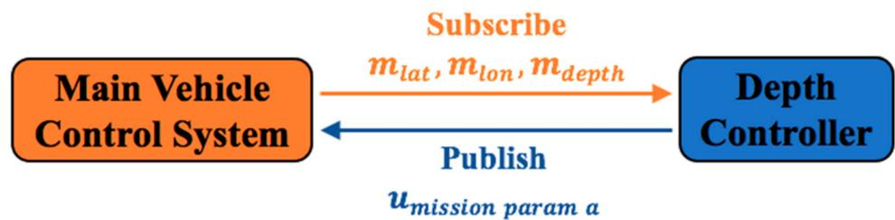
**Figure 10.** Exchange of data between the main vehicle control system and a depth controller when the glider changed its depth based on a simplified fluorescence field.
