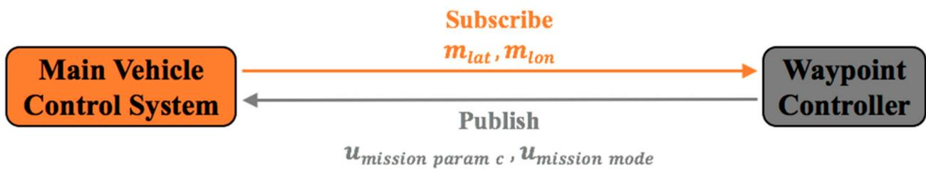
**Figure 21.** Exchange of data between the main vehicle control system and the waypoint controller when the glider changed its target points adaptively.
