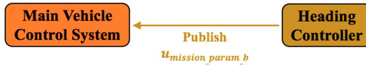
**Figure 14.** Exchange of data between the main vehicle control system and a heading controller when the glider followed a heading commanded by the backseat driver.
