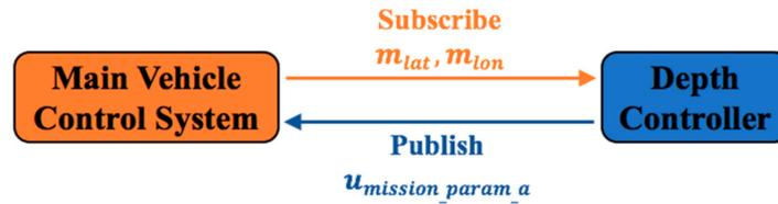
**Figure 7.** Exchange of data between the main vehicle control system and a depth controller when the glider changed its depth when a waypoint was reached.
