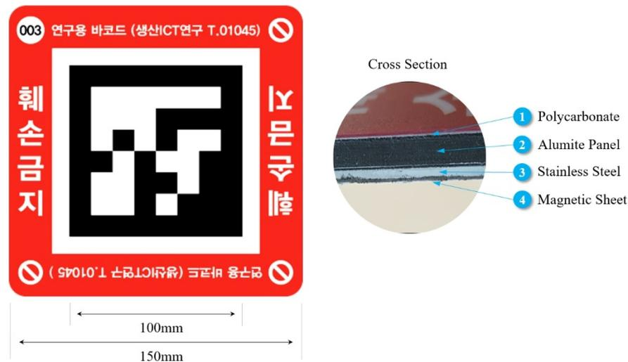
Figure 7. Design details of proposed marker.
