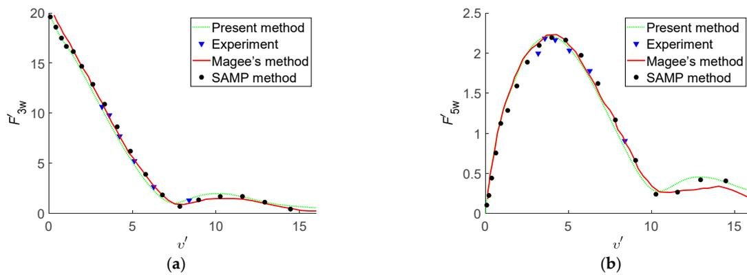
Figure 14. Non-dimensional wave exciting force amplitude at  $Fn = 0.2$ : (a) heave; (b) pitch.
