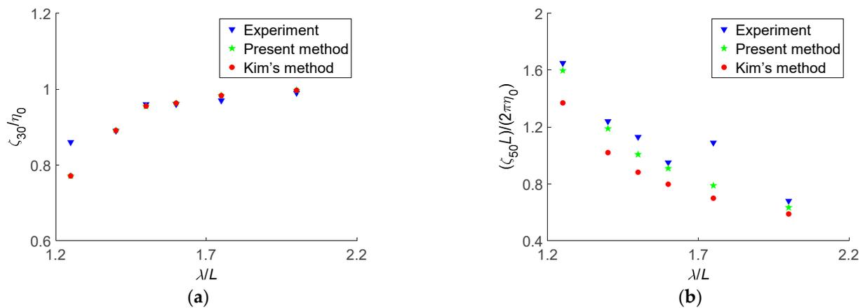
Figure 16. Response amplitude operators of motion for Wigley I hull at  $Fn = 0.2$  in head regular waves: (a) heave; (b) pitch.
