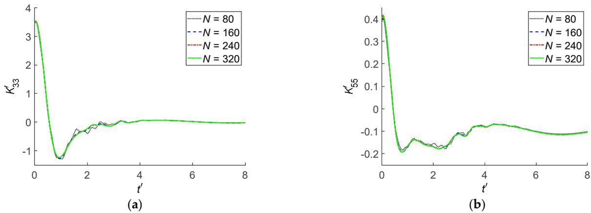
Figure 8. Non-dimensional memory function of Wigley I hull: (a) heave; (b) pitch.
