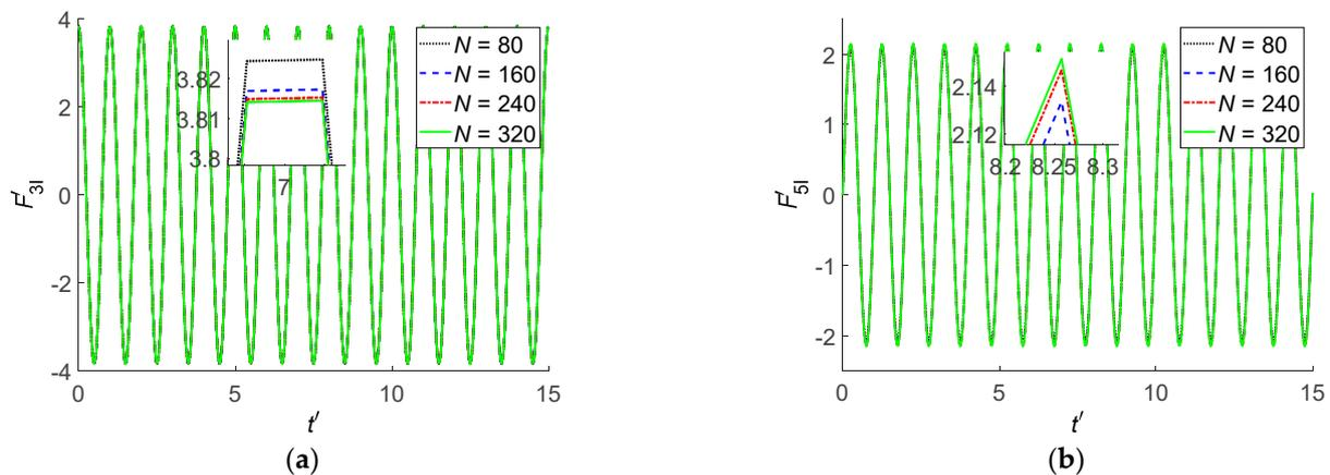
Figure 9. Non-dimensional F–K forces of Wigley I hull ( $\lambda/L = 1$ ): (a) heave; (b) pitch.
