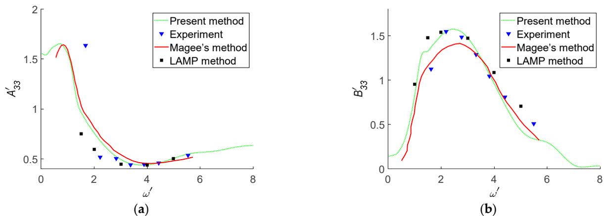
Figure 12. Non-dimensional heave-heave added mass and damping coefficients: (a)  $A'_{33}$ ; (b)  $B'_{33}$ .
