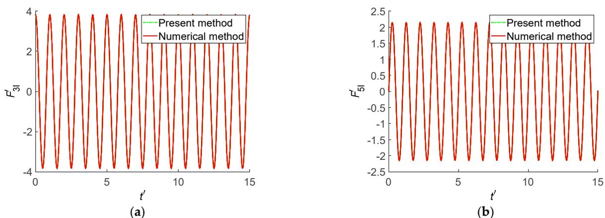
**Figure 10.** Time history of non-dimensional F-K forces of Wigley I hull obtained by “present method” and “numerical method” ( $\lambda/L = 1$ : (a) heave; (b) pitch).
