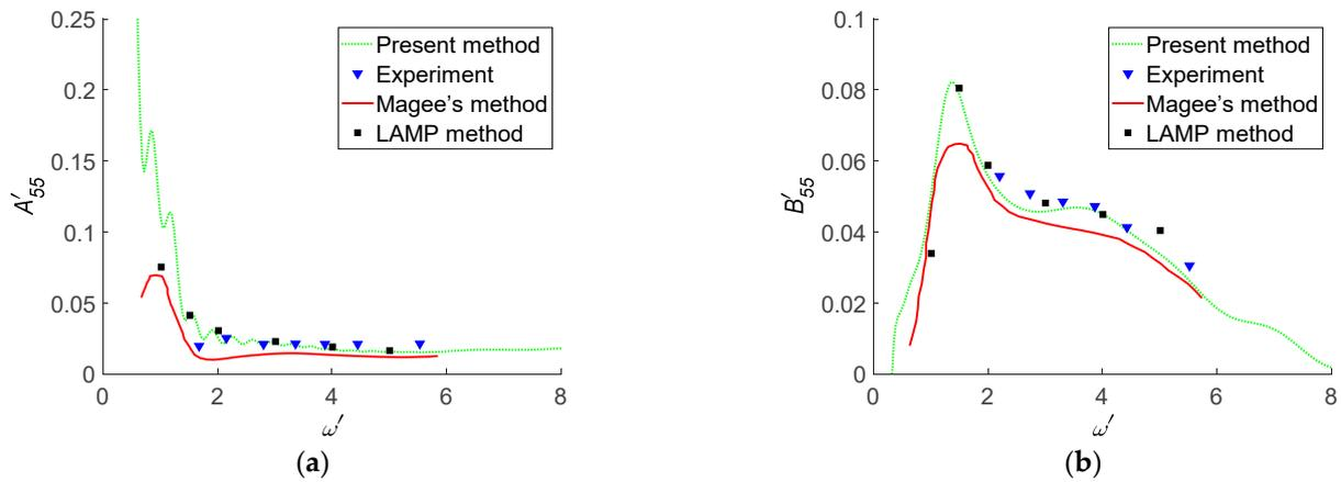
Figure 13. Non-dimensional pitch-pitch added mass and damping coefficients: (a)  $A'_{55}$ ; (b)  $B'_{55}$ .
