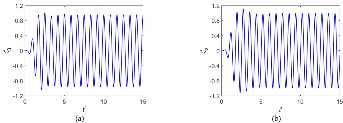
Figure 15. Non-dimensional time history of motions of Wigley I hull ( $\lambda/L = 1.5$ ): (a) heave; (b) pitch.
