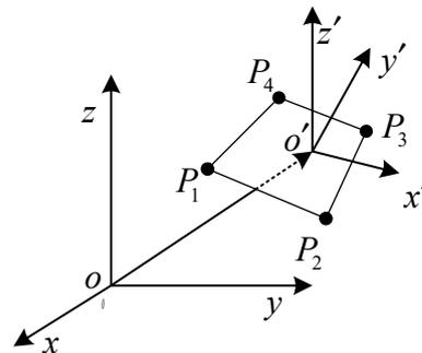
Figure 2. The reference coordinate system  $o-xyz$  and local panel coordinate system  $o'-x'y'z'$ .
