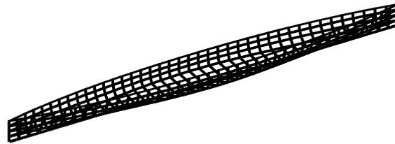
Figure 6. The panels’ distribution on the Wigley I hull.
