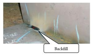
Figure 19. Bead backfill.
