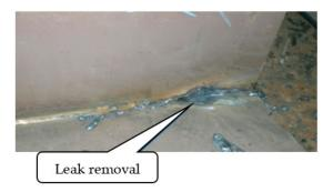
Figure 18. Piece leak removal.
