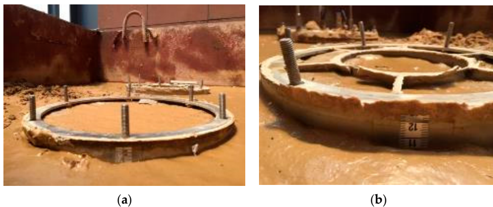
Figure 10. Soil plug in the penetration of the bucket foundation. (a) Mono-compartment bucket foundation; (b) Multi-compartment bucket foundation.
