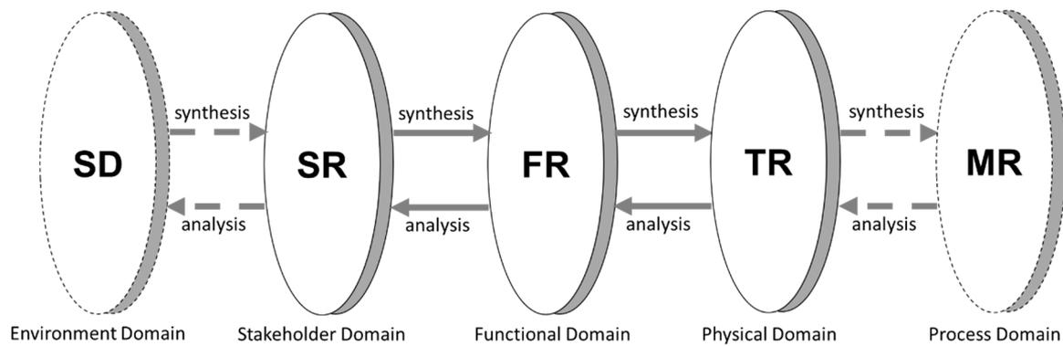
**Figure 1.** Domains of the design world (adapted from [49]). System Drivers (SD), stakeholder requirements (SR), functional requirements (FR), technical requirements (TR) and manufacturing requirements (MR).
