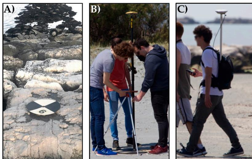
**Figure 3.** A numbered GCP in the survey area, made with high-density heavy plywood (A); GCP survey by means of NRTK technique (B); PPK survey performed by mounting the surveying system in a rigid backpack (C).
