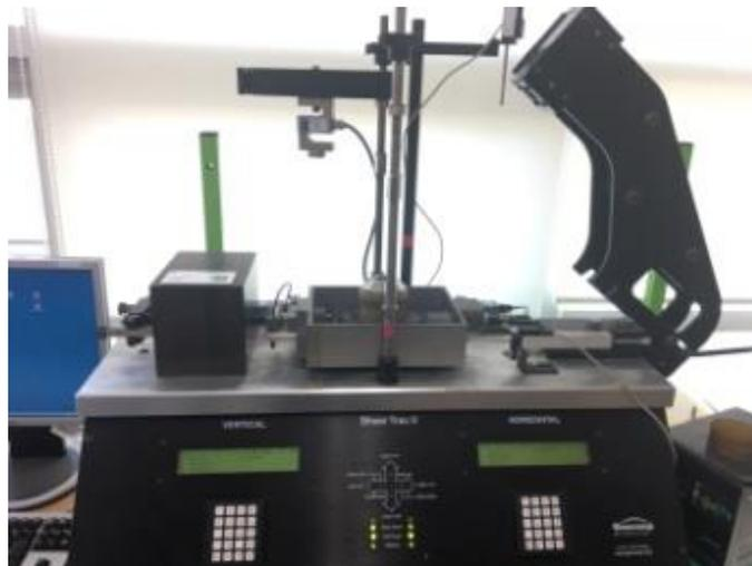
Figure 4. Direct simple shear apparatus.
