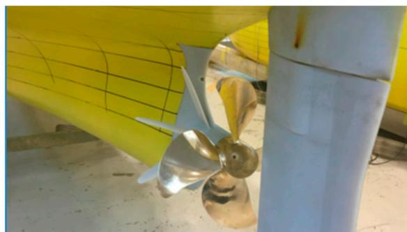
**Figure 17.** Propulsion test setup with the designed PSS.
