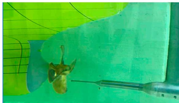
**Figure 16.** 3D wake measurements setup.
