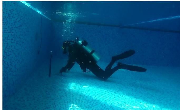
**Figure 4.** In experiment, one channel data acquisition system is used to record the diver’s breathing sound underwater. Sample rate is 50 kHz.
