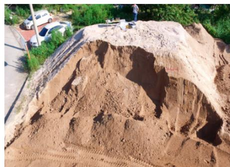
**Figure 7.** Slope failure after cutting.
