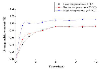
Figure 8. Variation curve of the average moisture content of red-bed sandstone at different temperatures.
