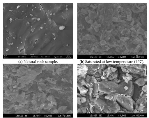
(c) Saturated at room temperature (23 °C). (d) Saturated at high temperature (45 °C).
