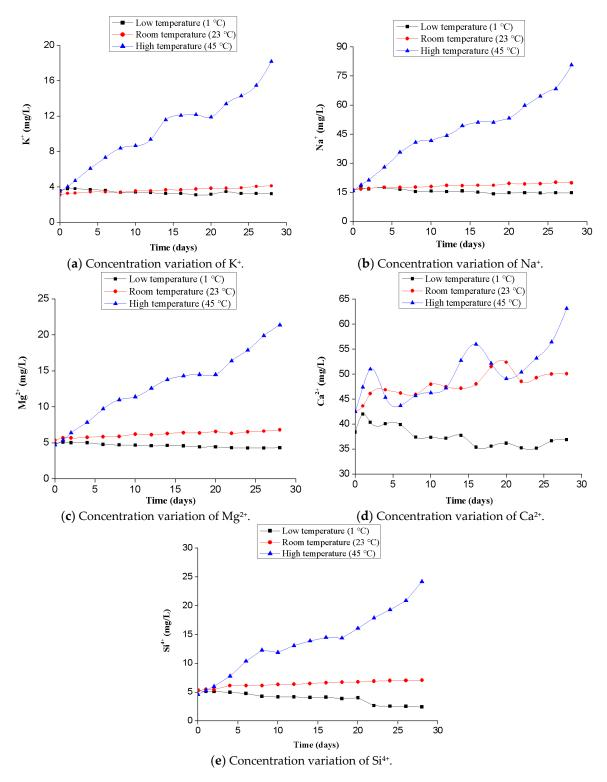
Figure 6. Curve of the main cationic concentration in the circulating aqueous solution at different temperatures.
