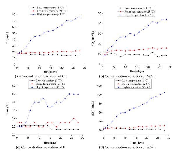
**Figure 7.** Curves of the concentration variation in the main anions in the circulating aqueous solution at different temperatures.
