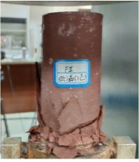
(**b**) Rock sample under low-temperature immersion.
