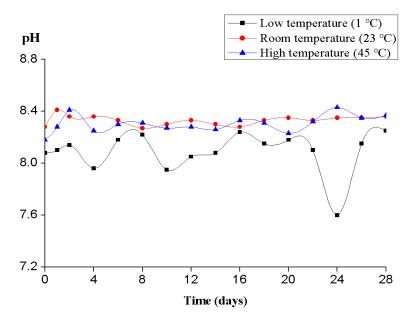
**Figure 5.** Change diagram of the pH of the circulating aqueous solution in turbulent flow at different temperatures. Changes in the main anodic and cationic concentrations.
