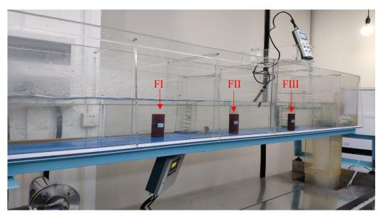
Figure 4. State diagram of the low-temperature (1 °C) test under dynamic water conditions.
