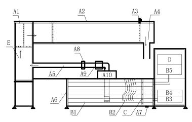
Figure 1. Structural schematic diagram of multifunctional open channel hydraulics test equipment.
