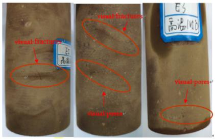
(a) High-temperature test specimens.
