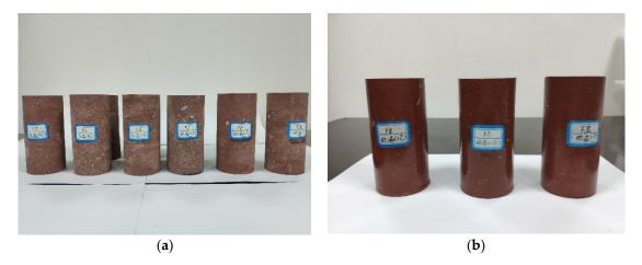
Figure 3. Sample chart: (a) Natural rock sample; (b) Saturated rock sample.
