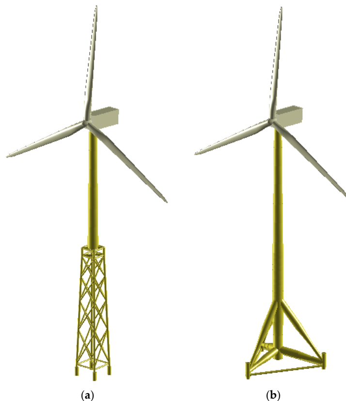
Figure 1. Test structures: (a) Jacket; (b) Tripod.
