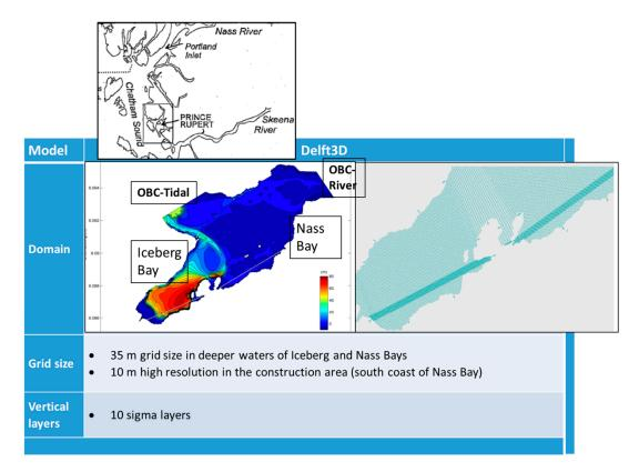
**Figure 11.** The model domain, including water depths and the horizontal grids, for the Delft3D sediment transport model used to simulate the fate and transport of sediments from trenching and backfilling for marine pipeline construction in Nass Bay.
