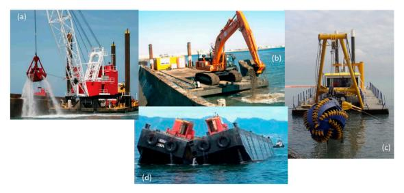
**Figure 6.** Examples of marine construction equipment: (**a**) A clamshell bucket grab; (**b**) a barge-mounted backhoe; (**c**) a cutter suction head and support vessel; and (**d**) a split hull barge used for disposal at sea.
