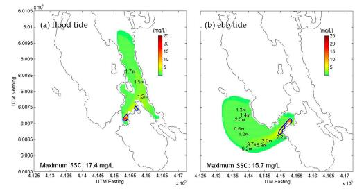
**Figure 8.** Model-derived suspended sediment concentration (SSC) (mg/L above background, maximum value in the water column) for (**a**) a flood tide and (**b**) and ebb tide. Numbers mark depths (above seabed) of maximum values in vertical column. Blue contours present the areas of SSC greater than 5 mg/L.
