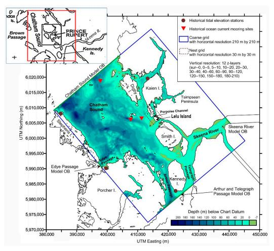
**Figure 7.** The model domain, open boundaries (OB), water depths and locations of current meter data sets used in model verification for the numerical sediment transport model for dredging in Porpoise Channel.
