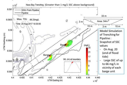
**Figure 12.** Model derived simulations of suspended sediment concentrations for trenching of the Nass Bay pipeline by two clamshell dredge units.
