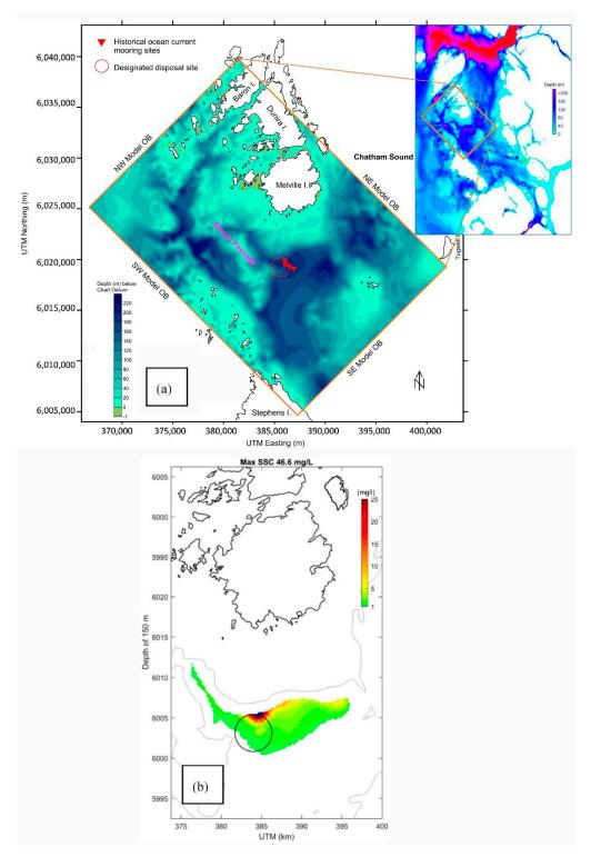
**Figure 10.** (a) The Brown Passage model domain and its water depths and (b) a sample of the model results for the sediment plume at 150 m depth realized from the disposal at sea operations. Areas with SSC greater than 25 mg/L are marked by blue color. The black circle marks a previously used ocean disposal site (1 nautical mile in diameter).
