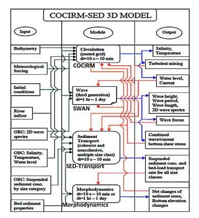
**Figure 4.** Schematic diagram of the COastal CIRculation and SEDiment transport Model (COCIRM-SED) numerical model. OBC represents Open Boundary Conditions, SWAN is the Simulating WAves Nearshore ocean wave model [12] and dt is the user-selectable time scale range for which bottom elevations are adjusted in the Morphodynamics module.
