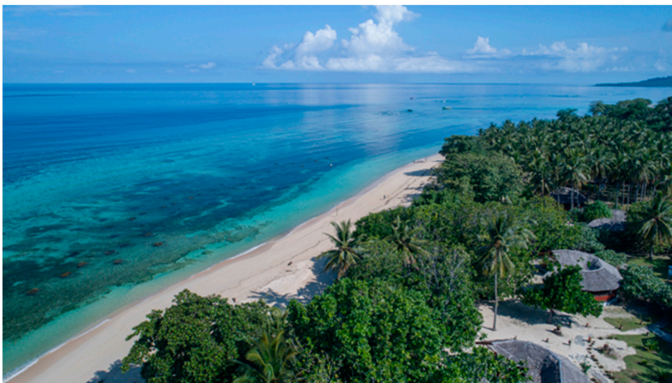
Figure 3. Soon after start of the project, at low tide (wide angle image). The tops of the reef restoration structures are clearly visible. The eroded curve is the area where the beach grew back.
